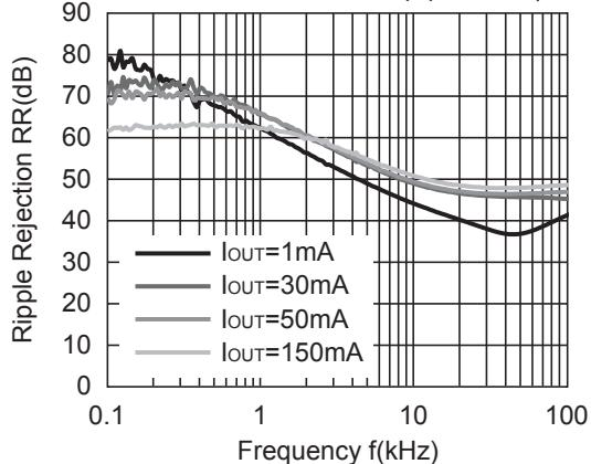
**R1116x401x** $V_{IN}=5V_{DC}+0.5V_{p-p}, C_{OUT}=2.2\mu F$
