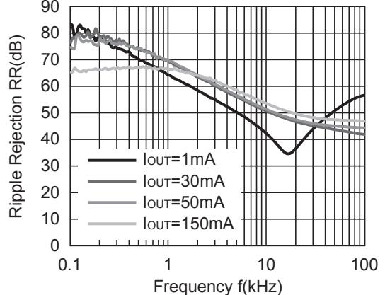
**R1116x401x** $V_{IN}=5V_{DC}+0.5V_{p-p}, C_{OUT}=1\mu F$
