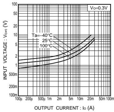
Fig.9 Input voltage vs. output current (ON characteristics)
