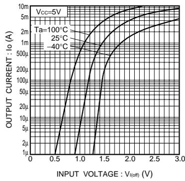
Fig.10 Output current vs. input voltage (OFF characteristics)
