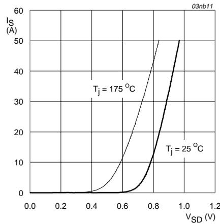
$V_{GS} = 0\text{ V}$
