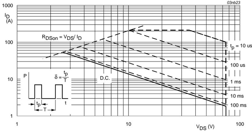
T<sub>mb</sub> = 25 °C; I<sub>DM</sub> single pulse.
