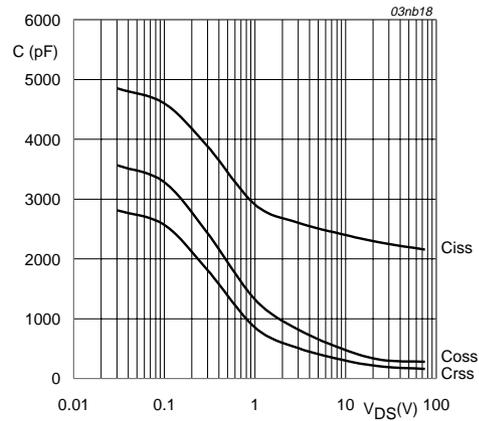
$V_{GS} = 0 \text{ V}; f = 1 \text{ MHz}$
