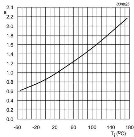
$$a = \frac{R_{Dson}}{R_{Dson(25^\circ\text{C})}}$$
