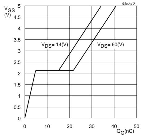
$T_j = 25^\circ\text{C}; I_D = 25\text{ A}$
