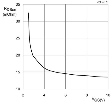
$T_j = 25^\circ\text{C}$ ;  $I_D = 25\text{ A}$
