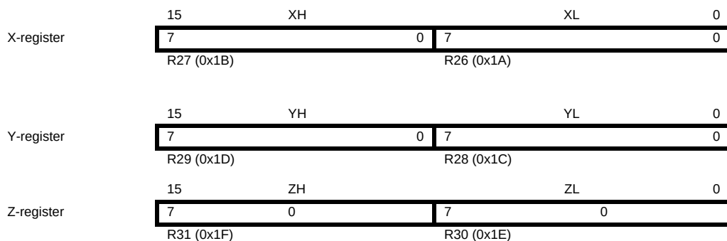
Figure 5. The X-, Y-, and Z-registers
