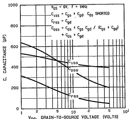
Fig. 10 — Typical Capacitance Vs.
