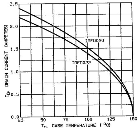
Fig. 13 — Maximum Drain Current Vs. Case Temperature
