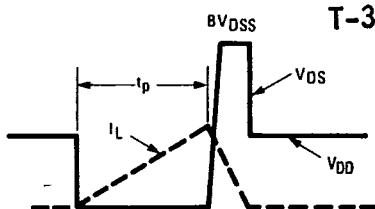
Fig. 15b — Unclamped Inductive Load Test Waveforms
