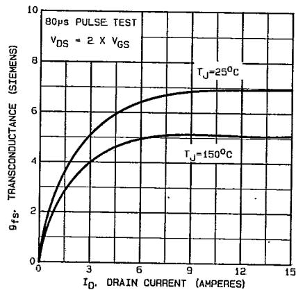
Fig. 6 — Typical Transconductance Vs. Drain Current
