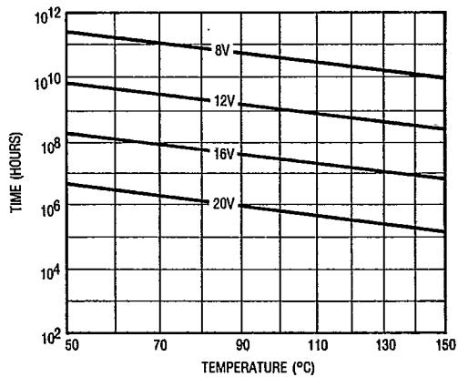
\*Fig. 18 — Typical Time to Accumulated 1% Gate Failure
