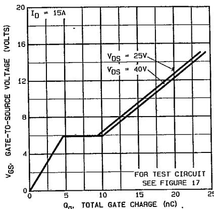
Fig. 11 — Typical Gate Charge Vs.
