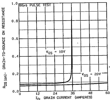
Fig. 12 — Typical On-Resistance Vs. Drain Current
