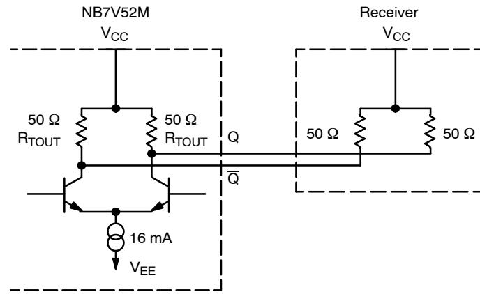
Figure 11. Typical CML Output Structure and Termination
