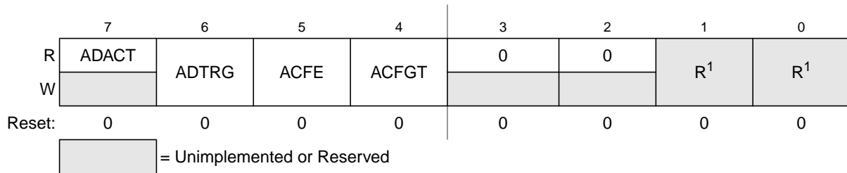
Figure 9-4. Status and Control Register 2 (ADCSC2)
