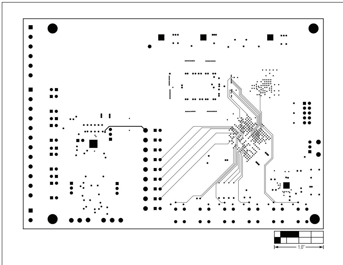
Figure 20. MAX11043 EV Kit PCB Layout—Signal Layer 9
