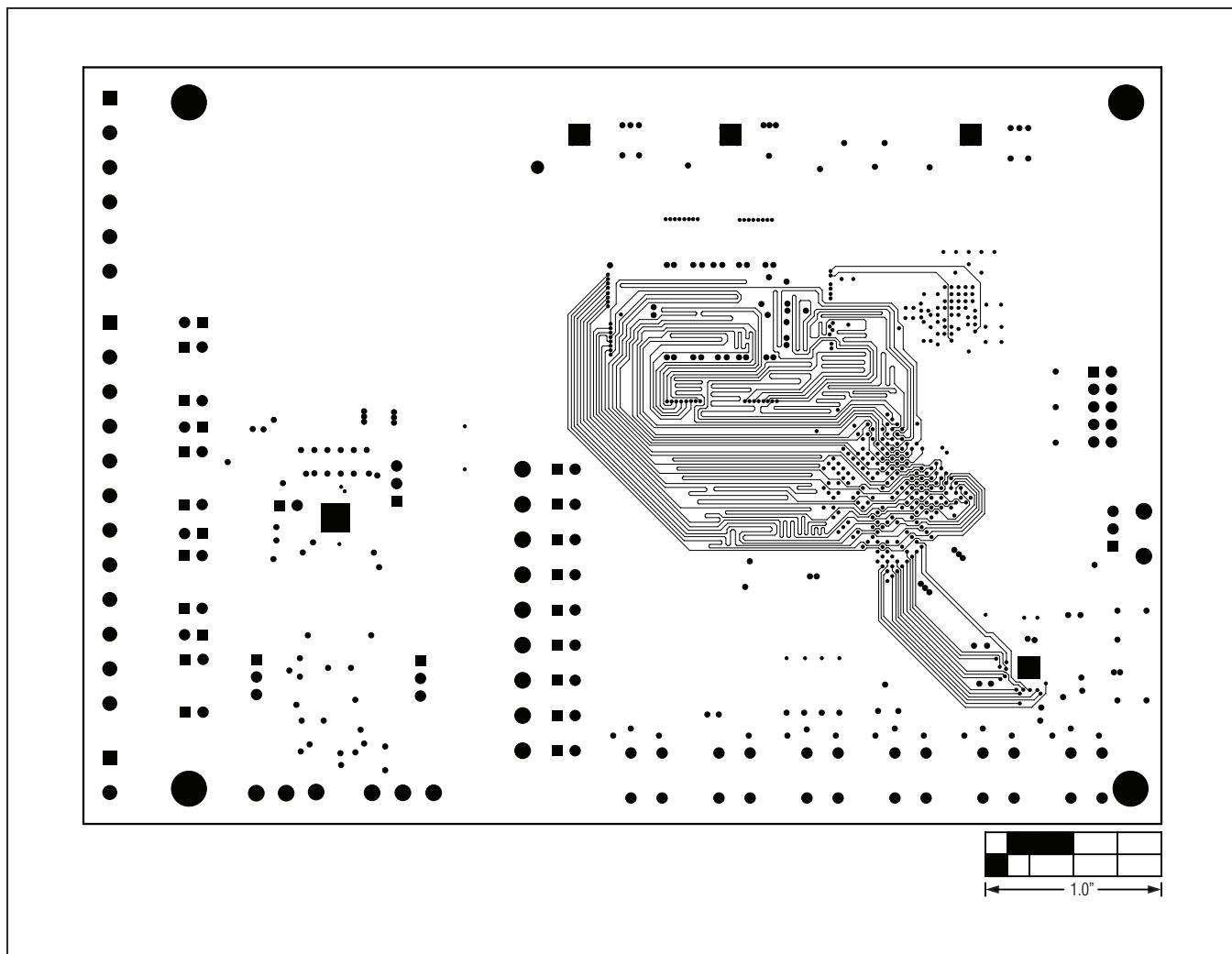
Figure 16. MAX11043 EV Kit PCB Layout—Power Layer 5
