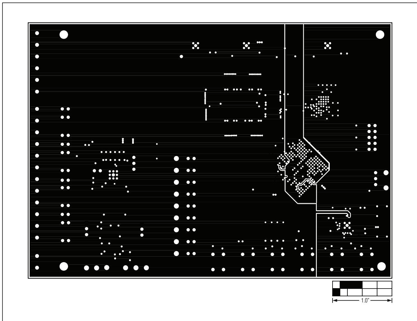
Figure 17. MAX11043 EV Kit PCB Layout—Signal Layer 6
