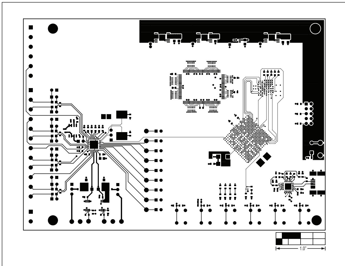
Figure 12. MAX1104311043 EV Kit PCB Layout—Component Side
