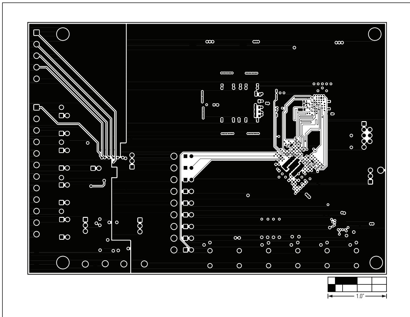
Figure 21. MAX11043 EV Kit PCB Layout—Solder Side
