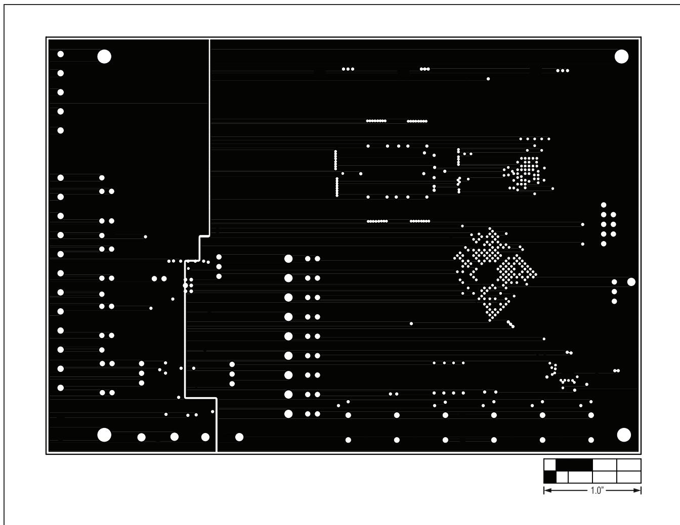
Figure 19. MAX11043 EV Kit PCB Layout—Ground Layer 8
