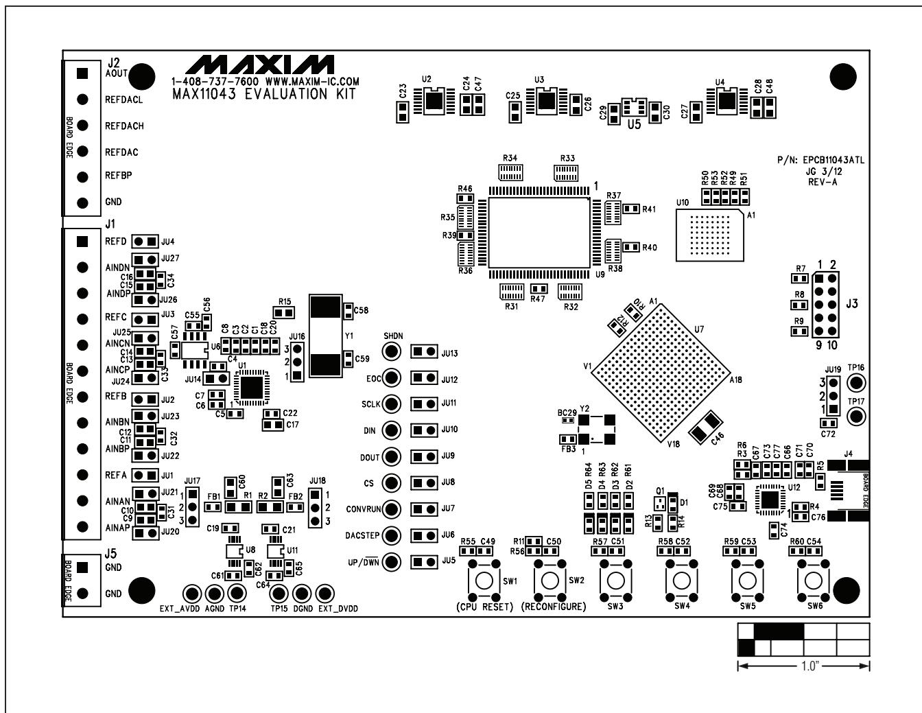
Figure 10. MAX11043 EV Kit Component Placement Guide—Component Side
