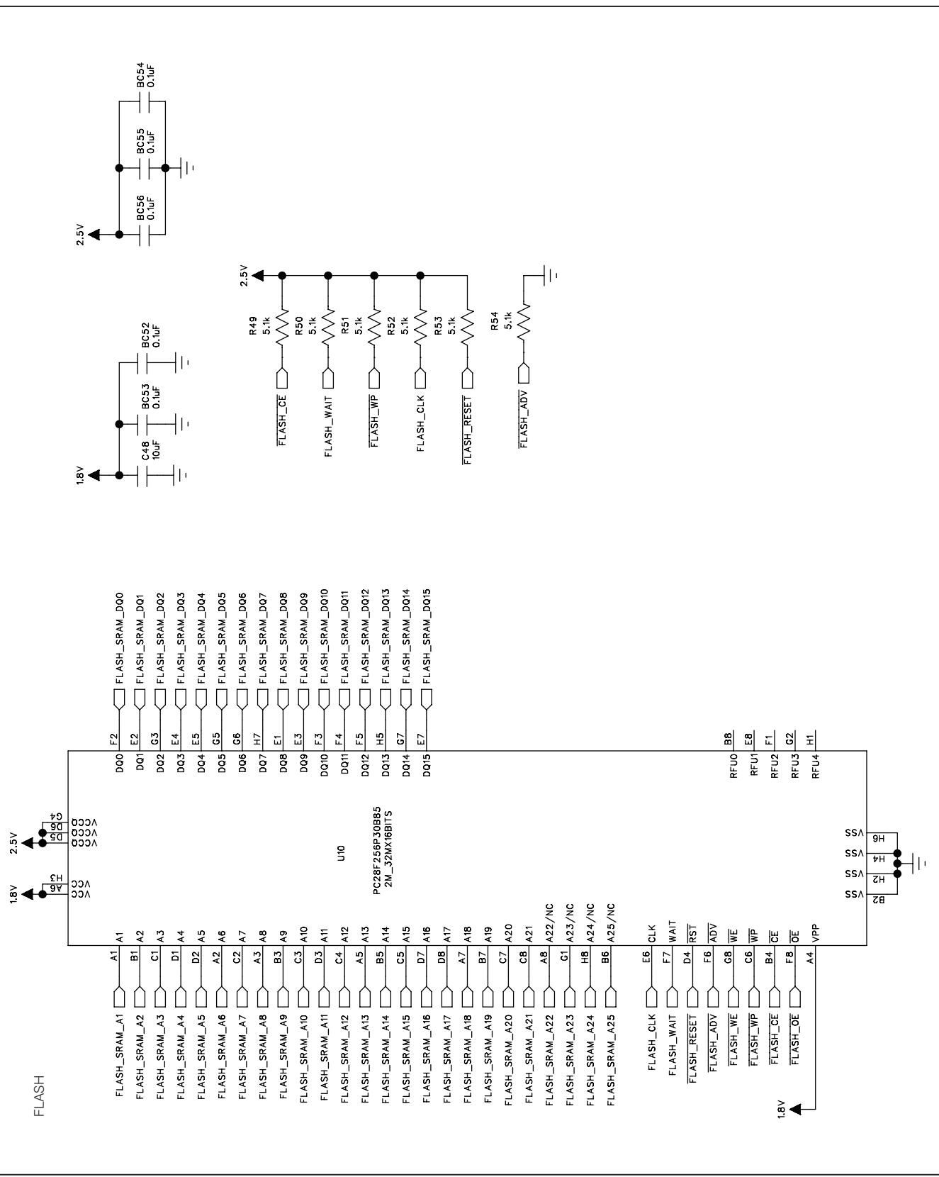
Figure 9i. MAX11043 EV Kit Schematic (Sheet 9 of 10)
