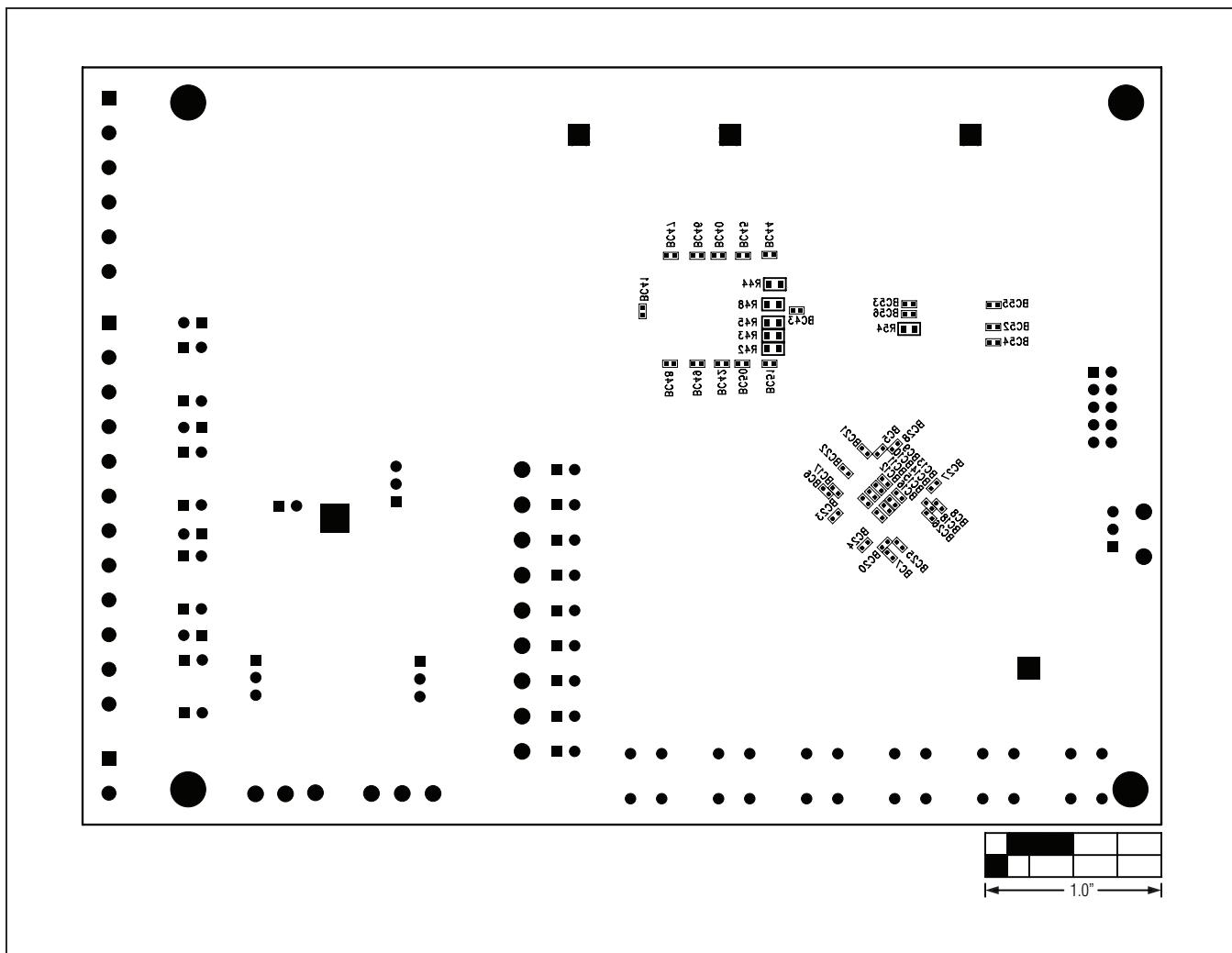
*Figure 11. MAX11043 EV Kit Component Placement Guide—Solder Side*
