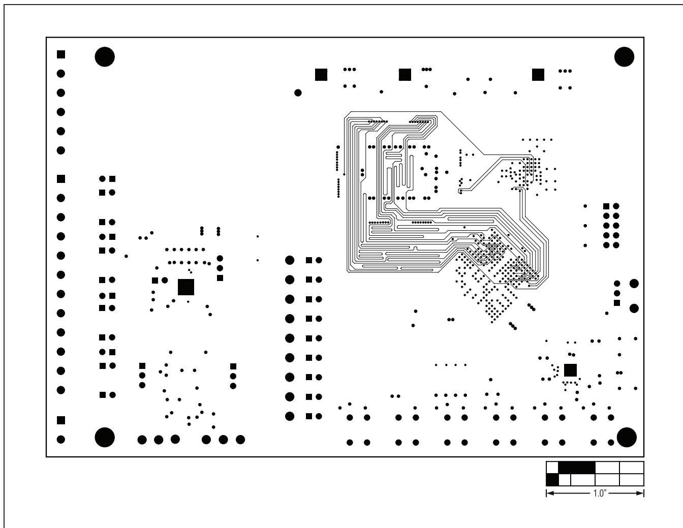
Figure 14. MAX11043 EV Kit PCB Layout—Signal Layer 3
