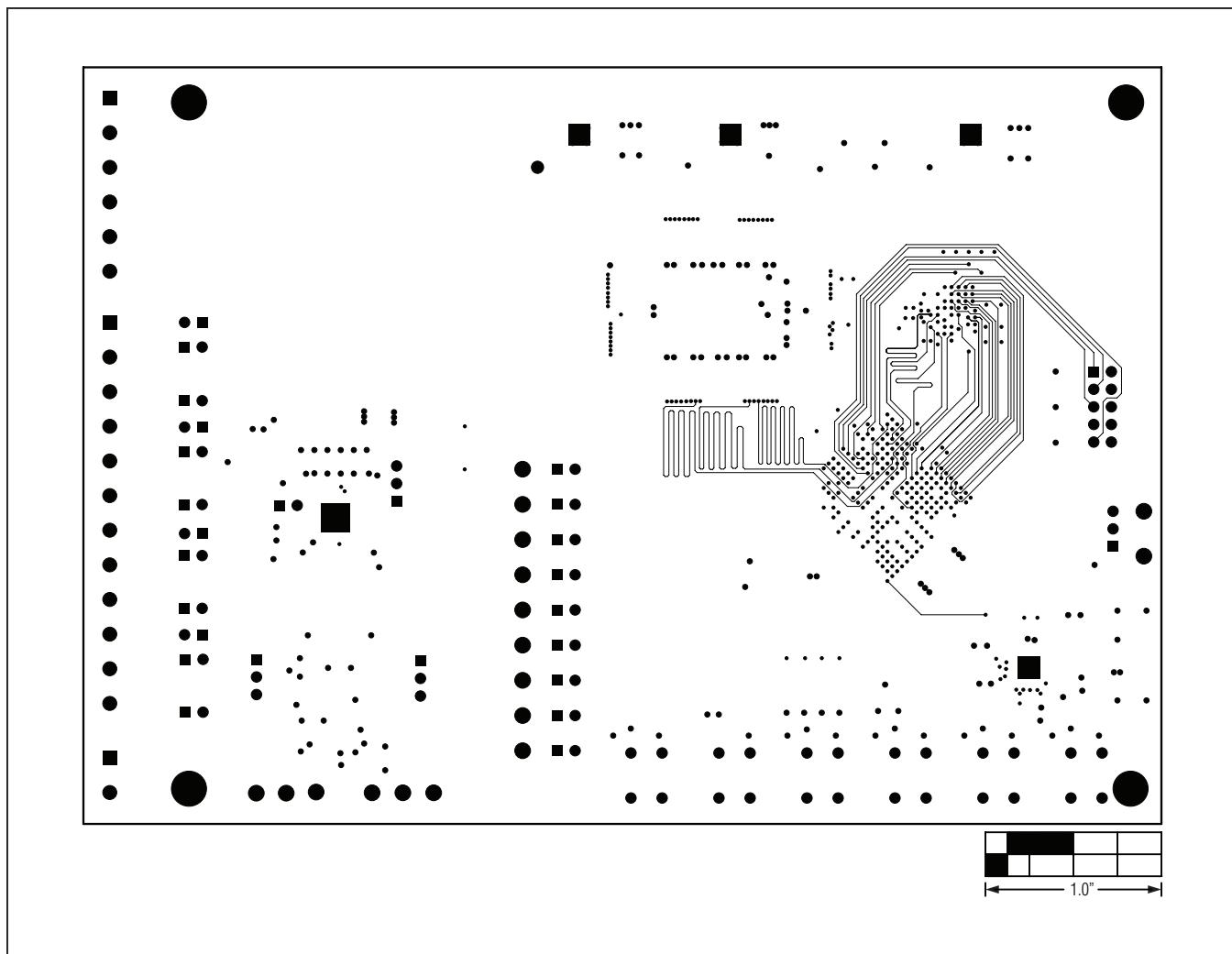
Figure 18. MAX11043 EV Kit PCB Layout—Ground Layer 7
