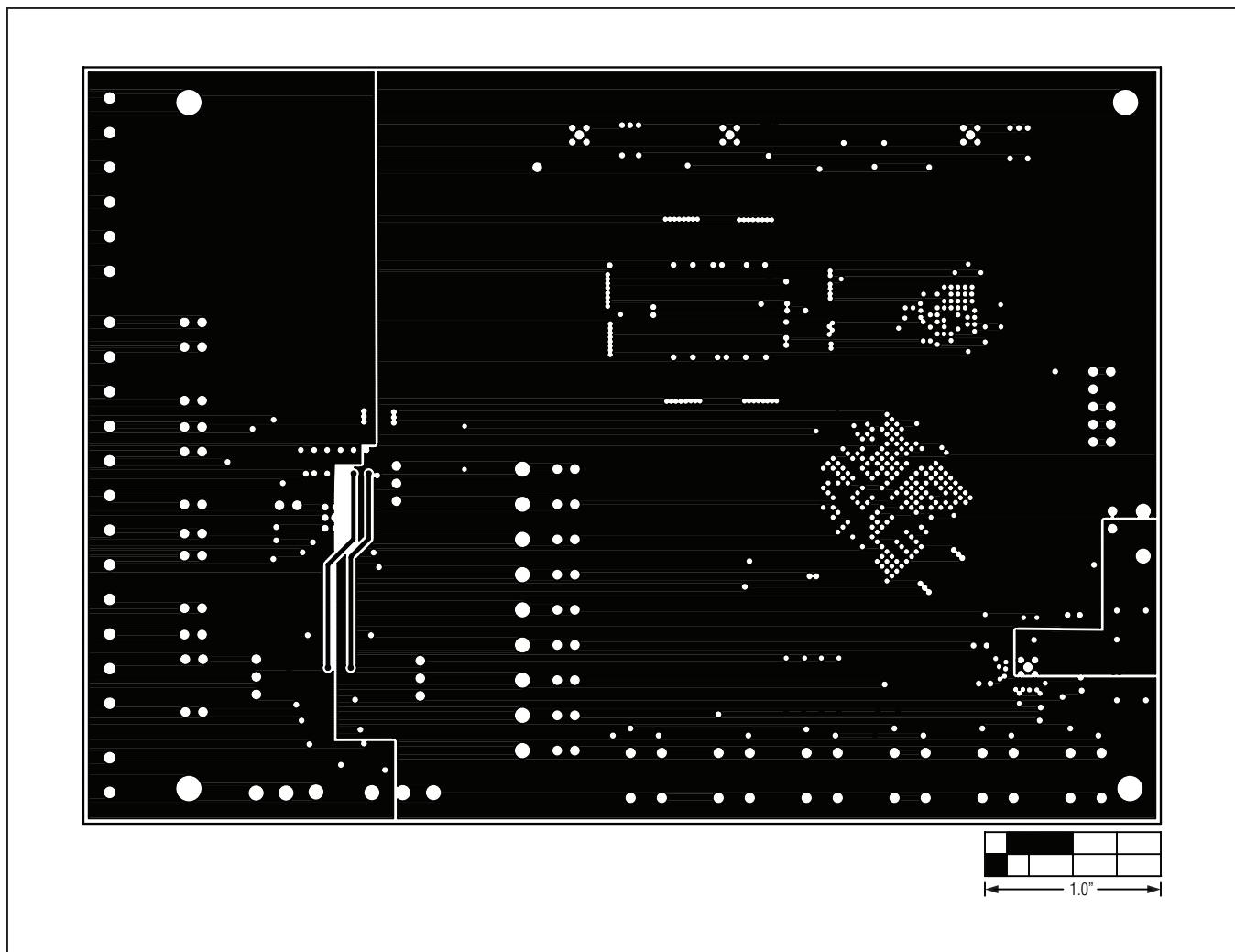
Figure 15. MAX11043 EV Kit PCB Layout—Ground Layer 4
