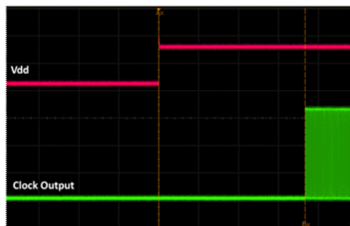
Figure 17. Startup Waveform vs. Vdd
