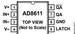
Figure 1. 8-Lead Narrow Body SOIC
