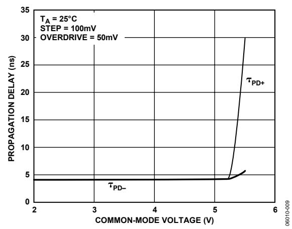
Figure 12. Propagation Delay vs. Common-Mode Voltage
