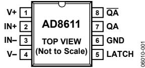
Figure 4. 8-Lead Narrow Body SOIC Pin Configuration
