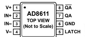
Figure 2. 8-Lead MSOP
