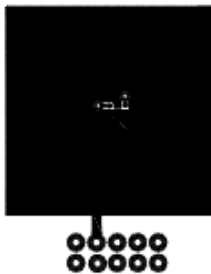
a. 52\text{ }^\circ\text{C/W} when mounted on a 1\ \text{in}^2 pad of 2 oz copper.
