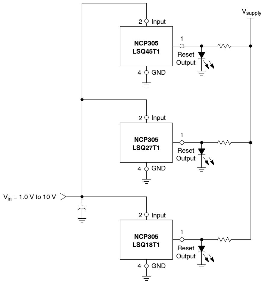
A simple voltage monitor can be constructed by connecting several voltage detectors as shown above. Each LED will sequentially turn on when the respective voltage detector threshold ( $V_{DET\_} + V_{HYS}$ ) is exceeded. Note that detector thresholds ( $V_{DET\_}$ ) that range from 0.9 V to 4.9 V in 100 mV steps can be manufactured.
