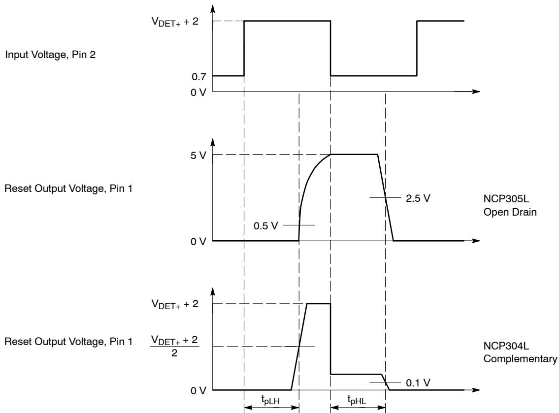
NCP304 and NCP305 series are measured with a 10 pF capacitive load. NCP305 has an additional 470 k pullup resistor connected from the reset output to +5.0 V. The reset output voltage waveforms are shown for the active low 'L' devices. The upper detector threshold,  $V_{DET+}$  is the sum of the lower detector threshold,  $V_{DET-}$  plus the input hysteresis,  $V_{HYS}$ .
