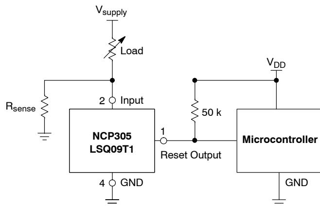
This circuit monitors the current at the load. As current flows through the load, a voltage drop with respect to ground appears across  $R_{sense}$  where  $V_{sense} = I_{load} * R_{sense}$ . The following conditions apply:
