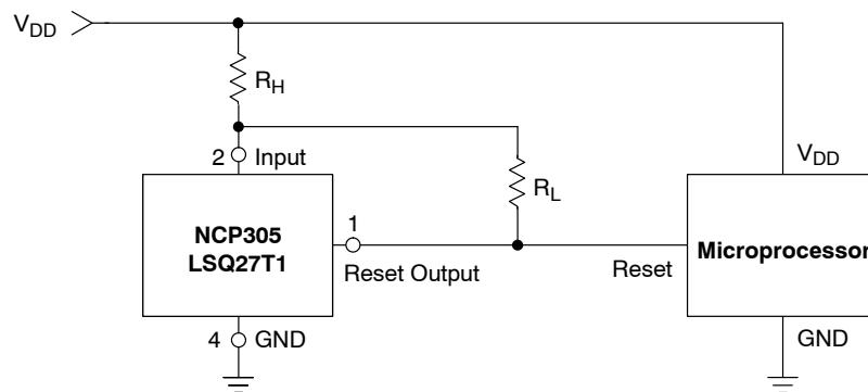
Figure 29. Microprocessor Reset Circuit with Additional Hysteresis
