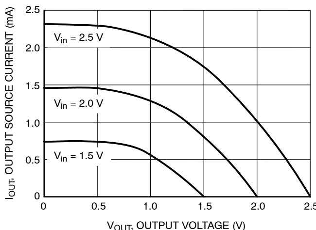
**Figure 13. NCP304H Series 2.7 V Reset Output
