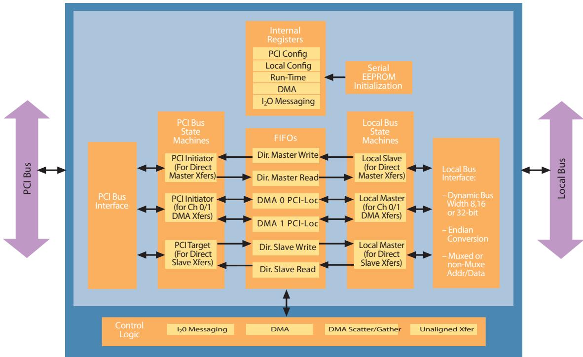
PCI 9054 Internal Block Diagram
