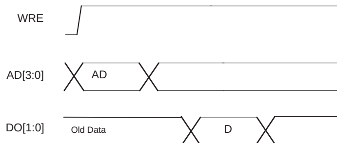
Figure 3-7. Slice Single /Dual Port Read Cycle Timing
