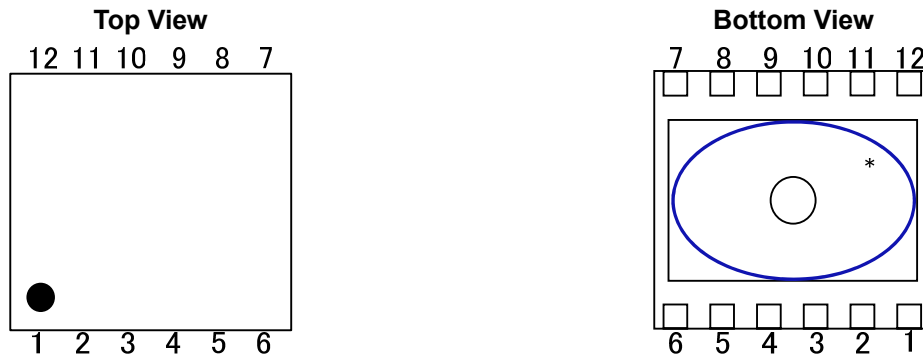
DFN(PLP)2730-12 Pin Configuration
