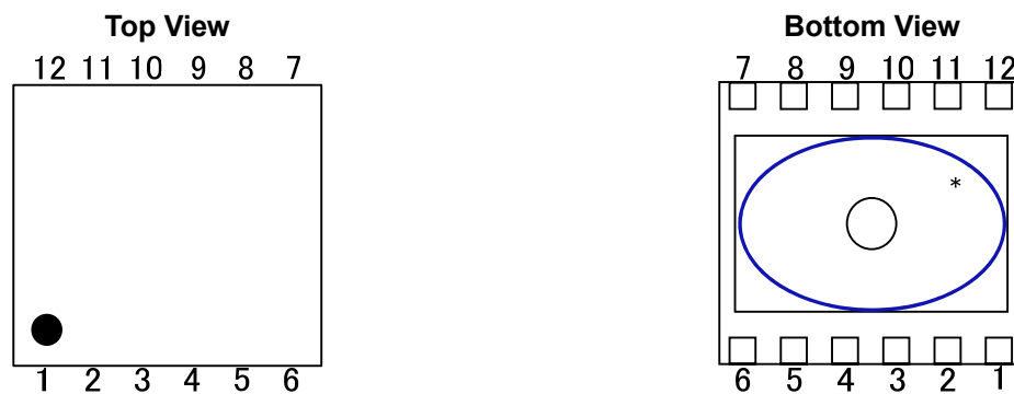
DFN(PLP)2730-12 Pin Configuration
