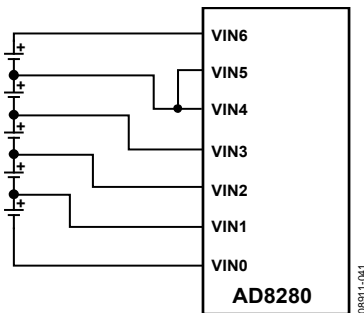
Figure 47. Five-Cell Connections for the AD8280
