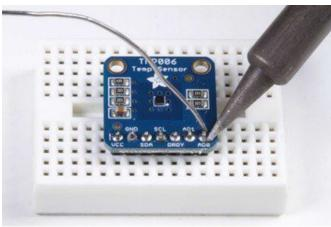
And Solder! Solder each pin for a solid electrical connection.
