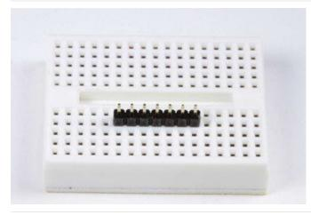
Position the Header Cut the header to length and insert it in a breadboard with the long pins down.
