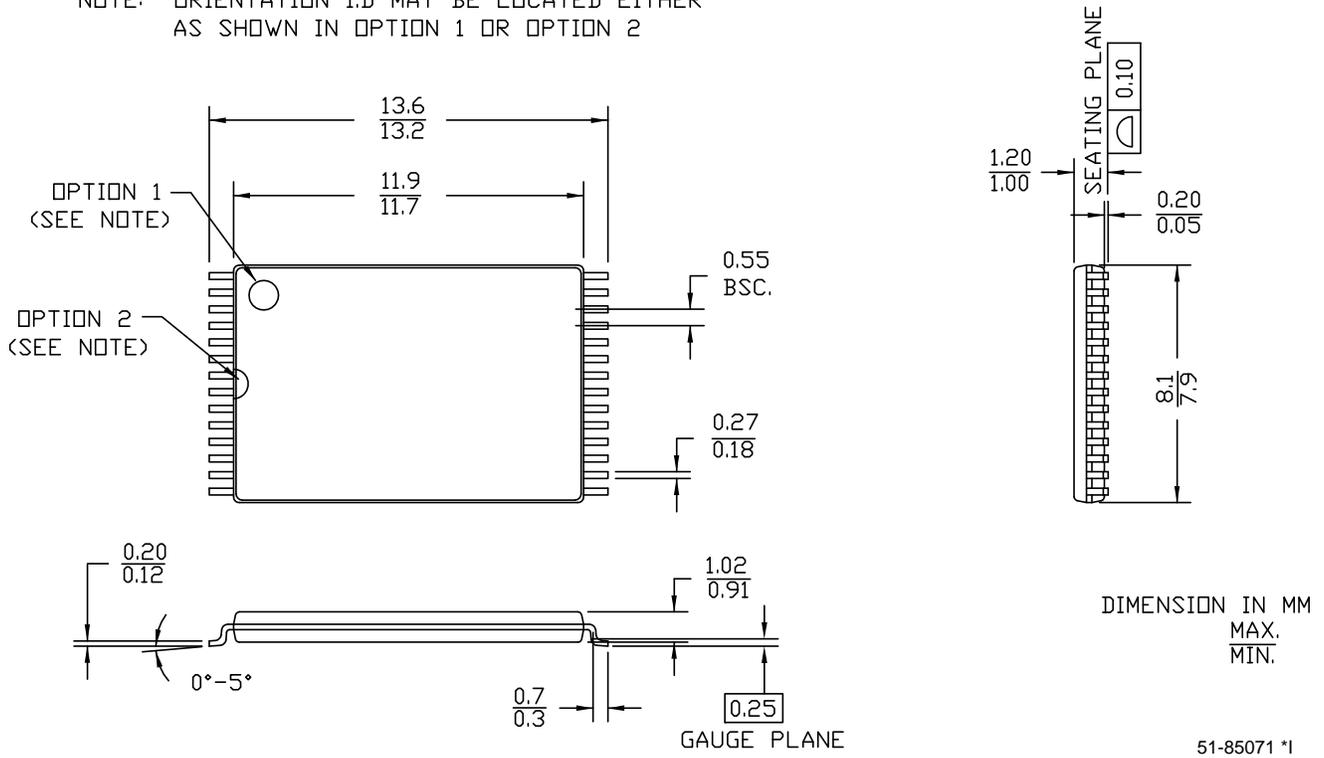
Figure 10. 28-pin Reverse TSOP 1 (8 x 13.4 mm), 51-85074
