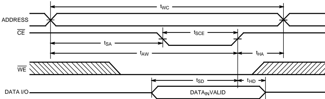
Figure 7. Write Cycle No. 3 ( $\overline{\text{WE}}$  Controlled,  $\overline{\text{OE}}$  LOW)<sup>[22, 23]</sup>
