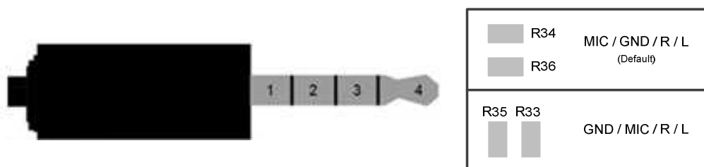
Figure 2 Headset Jack Configuration Options
