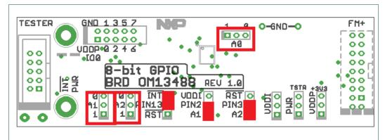
Fig 3. Jumper configuration for PCA8574, PCA8574A, PCA9534, PCA9554A, PCA9554B, PCA9554C, PCA9554, PCA9674A, PCA9674, PCAL9554B, PCAL9554C, PCF8574, PCF8574A
