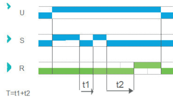
Function At - Summation time relay
