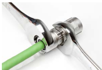
Step 16 - Tighten to 5-7 N/M using 25mm wrench
