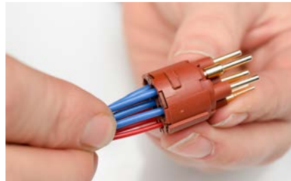
Step 7 - Push the contact holder into the sleeve
