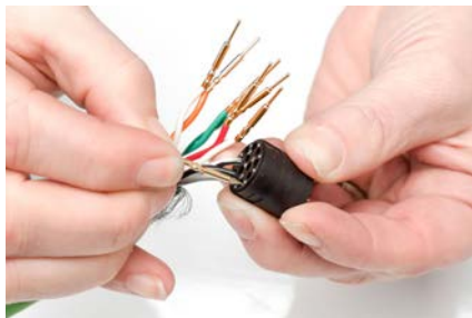
Step 7 - Push the contacts into the insert as required
