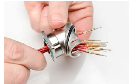
Step 4 - Crimp contacts onto wire
