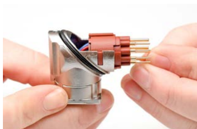
Step 9 - Place sub-assembly into shell
