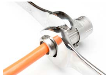
Step 17 - Tighten to 5-7 N/M using 25mm wrench
