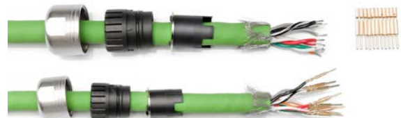
Step 6 - Crimp a contact onto each wire
