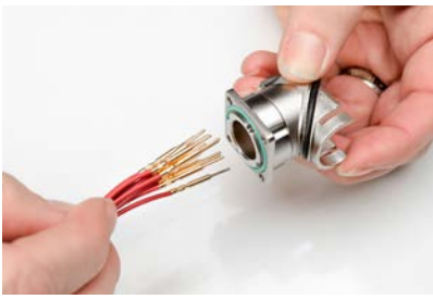
Step 3 - Slide wires through shell
