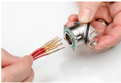
Step 3 - Slide wires through shell
