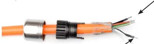
Step 5b - Strip signal wire 4.5mm
