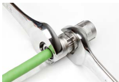
Step 16 - Tighten to 5-7 N/M using 25mm wrench
