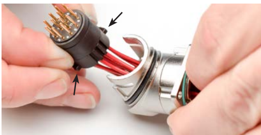
Step 5 - Locate keys on sides of insert
