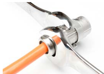
Step 17 - Tighten to 5-7 N/M using 25mm wrench
