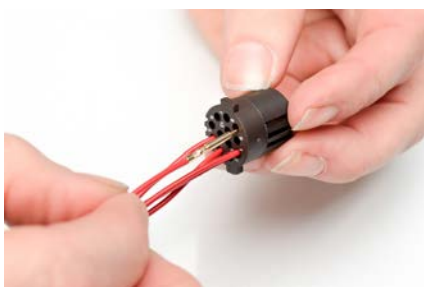
Step 4 - Push wire into insert
