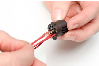
Step 4 - Push wire into insert
