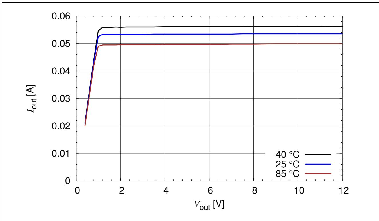
Figure 3-17 BCR321U: Output Current versus  $V_{\text{out}}$   $I_{\text{out}} = f(V_{\text{out}})$ ,  $V_{\text{EN}} = 3.3 \text{ V}$ ,  $R_{\text{ext}} = 20 \Omega$ ,  $T_A = \text{Parameter}$
