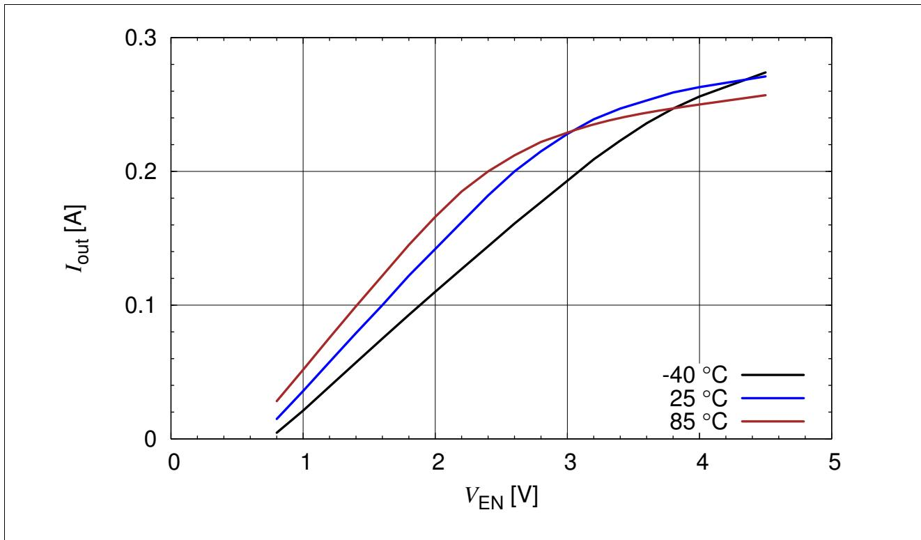
Figure 3-21 BCR321U: Output Current versus  $V_{EN}$   $I_{out} = f(V_{EN})$ ,  $V_{out} = 2$  V,  $R_{ext} = 3$  Ω,  $T_A$  = Parameter
