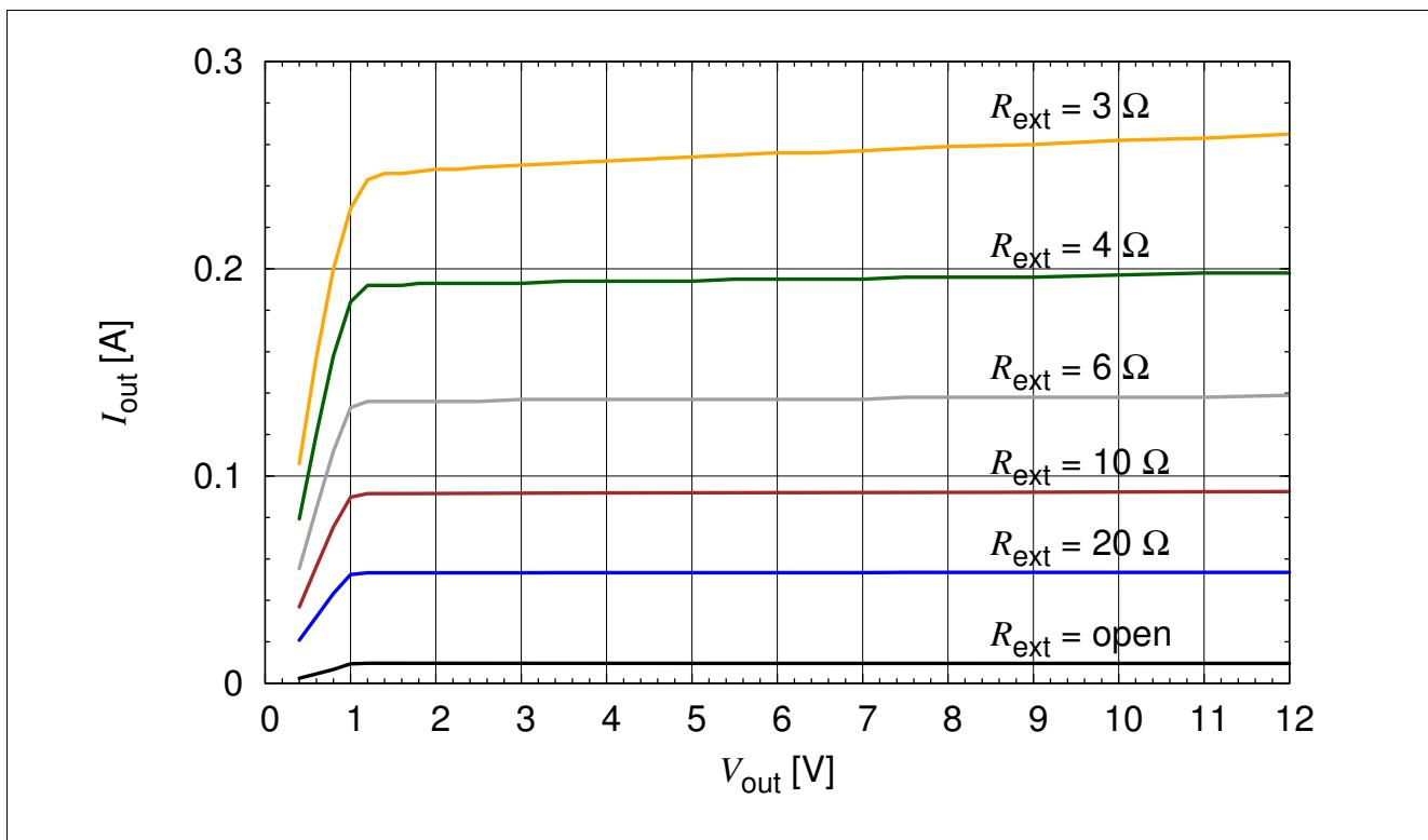
Figure 3-14 BCR321U: Output Current versus  $V_{\text{out}}$   $I_{\text{out}} = f(V_{\text{out}})$ ,  $V_{\text{EN}} = 3.3 \text{ V}$ ,  $R_{\text{ext}} = \text{Parameter}$
