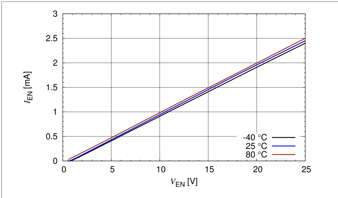
Figure 3-13 BCR320U: Enable Current versus  $V_{EN}$   $I_{EN} = f(V_{EN})$ ,  $R_{ext}$  = open,  $I_{out} = 0$  A,  $T_A$  = Parameter
