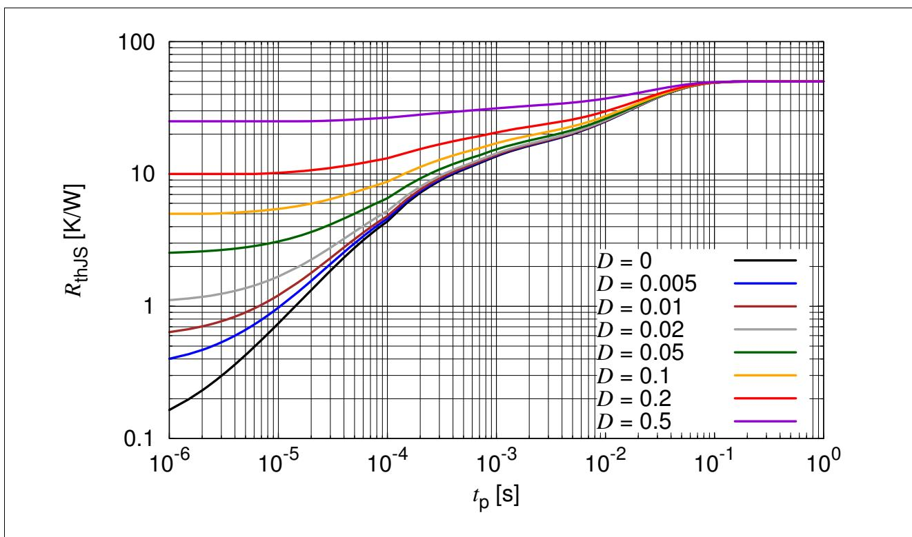
Figure 3-2 Permissible Pulse Load  $R_{\text{thJS}} = f(t_p)$
