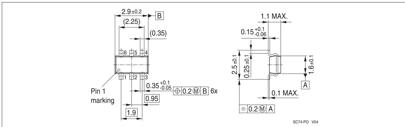
**Figure 5-1 Package Outline for SC74 (dimensions in mm)**
