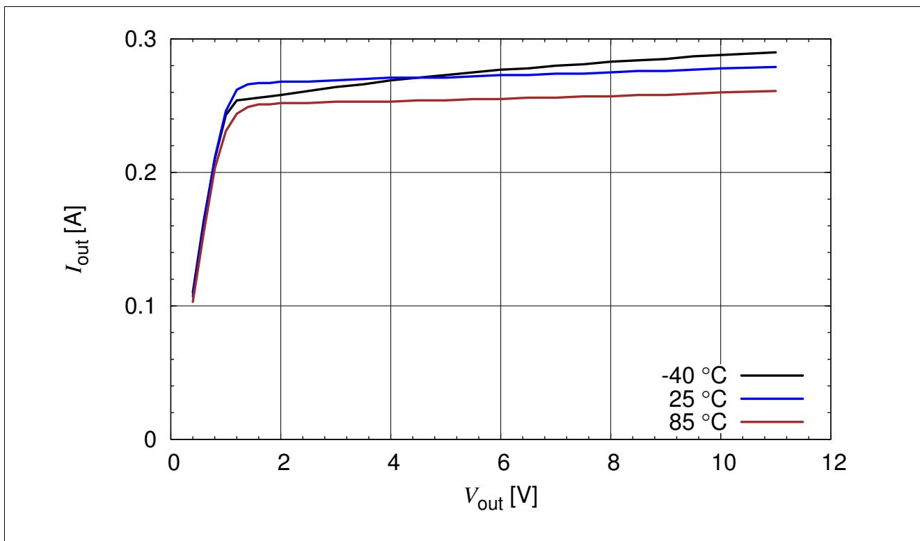
Figure 3-8 BCR320U: Output Current versus  $V_{\text{out}}$   $I_{\text{out}} = f(V_{\text{out}})$ ,  $V_{\text{EN}} = 12 \text{ V}$ ,  $R_{\text{ext}} = 3 \Omega$ ,  $T_A = \text{Parameter}$
