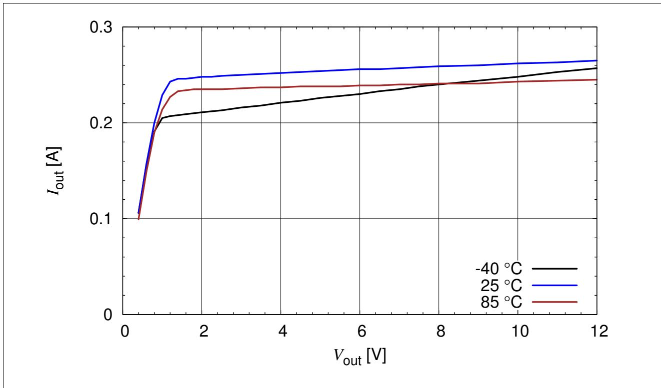
Figure 3-18 BCR321U: Output Current versus  $V_{\text{out}}$   $I_{\text{out}} = f(V_{\text{out}})$ ,  $V_{\text{EN}} = 3.3$  V,  $R_{\text{ext}} = 3$  Ω,  $T_A$  = Parameter
