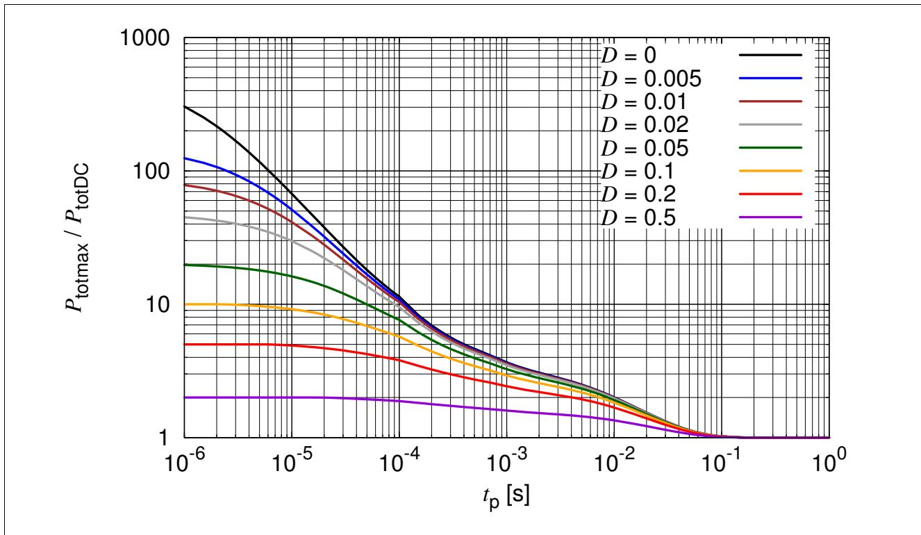
Figure 3-3 Permissible Pulse Load  $P_{\text{totmax}} / P_{\text{totDC}} = f(t_p)$
