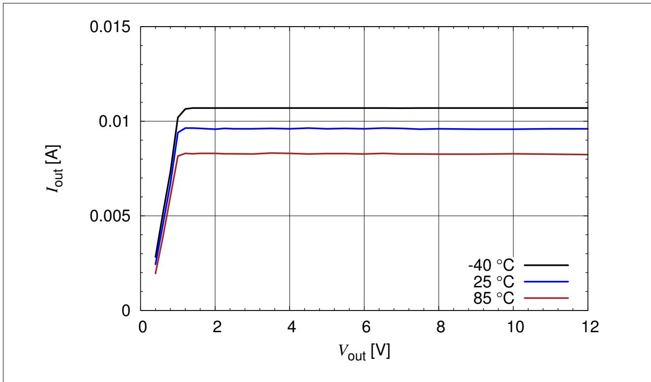
Figure 3-16 BCR321U: Output Current versus  $V_{\text{out}}$   $I_{\text{out}} = f(V_{\text{out}})$ ,  $V_{\text{EN}} = 3.3 \text{ V}$ ,  $R_{\text{ext}} = \text{open}$ ,  $T_A = \text{Parameter}$
