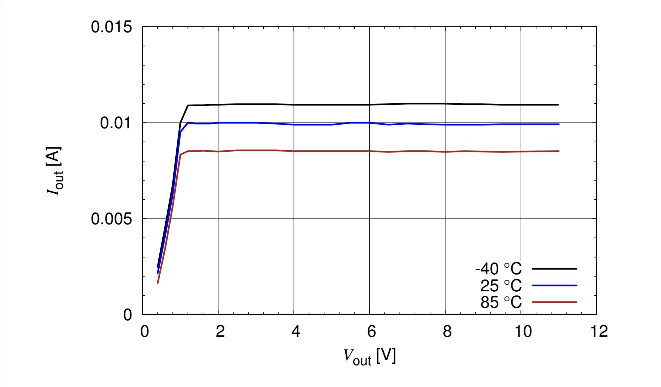
Figure 3-6 BCR320U: Output Current versus  $V_{\text{out}}$   $I_{\text{out}} = f(V_{\text{out}})$ ,  $V_{\text{EN}} = 12 \text{ V}$ ,  $R_{\text{ext}} = \text{open}$ ,  $T_A = \text{Parameter}$
