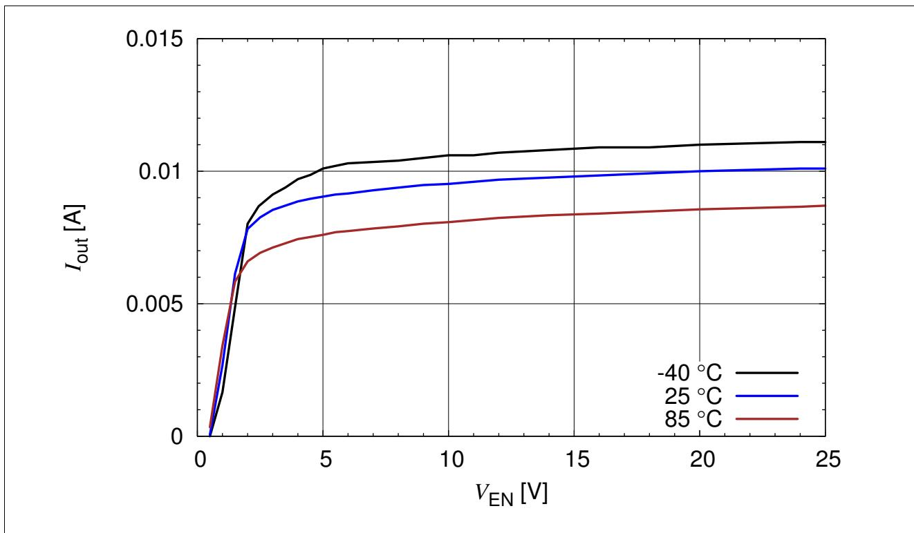
Figure 3-9 BCR320U: Output Current versus  $V_{\text{EN}}$   $I_{\text{out}} = f(V_{\text{EN}})$ ,  $V_{\text{out}} = 2 \text{ V}$ ,  $R_{\text{ext}} = \text{open}$ ,  $T_A = \text{Parameter}$
