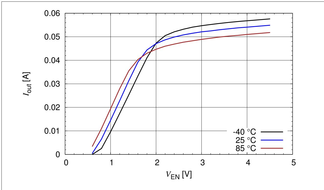
Figure 3-20 BCR321U: Output Current versus  $V_{EN}$   $I_{out} = f(V_{EN})$ ,  $V_{out} = 2$  V,  $R_{ext} = 20$  Ω,  $T_A$  = Parameter
