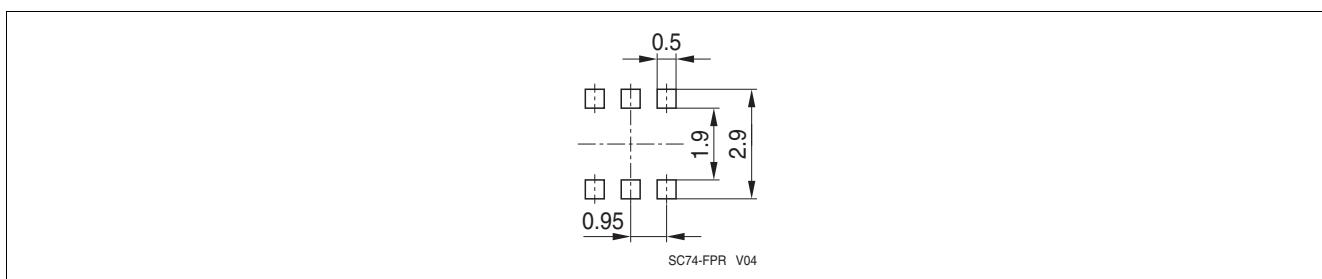
**Figure 5-2 Package Footprint for SC74 (dimensions in mm)**
