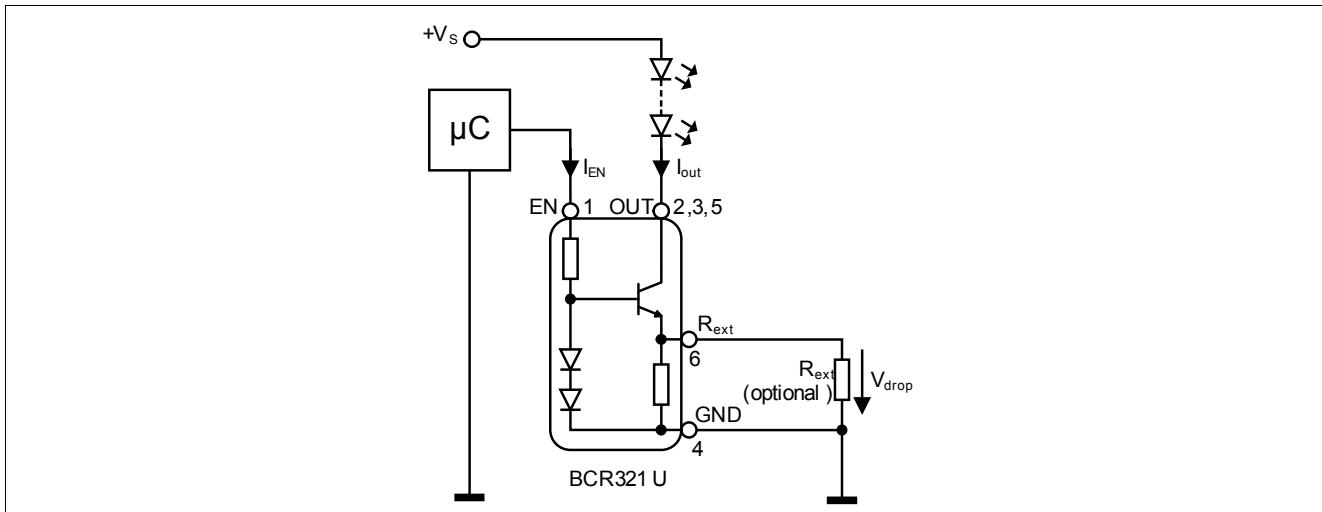
Figure 4-1 Application Circuit: Enabling / PWM by Micro Controller
