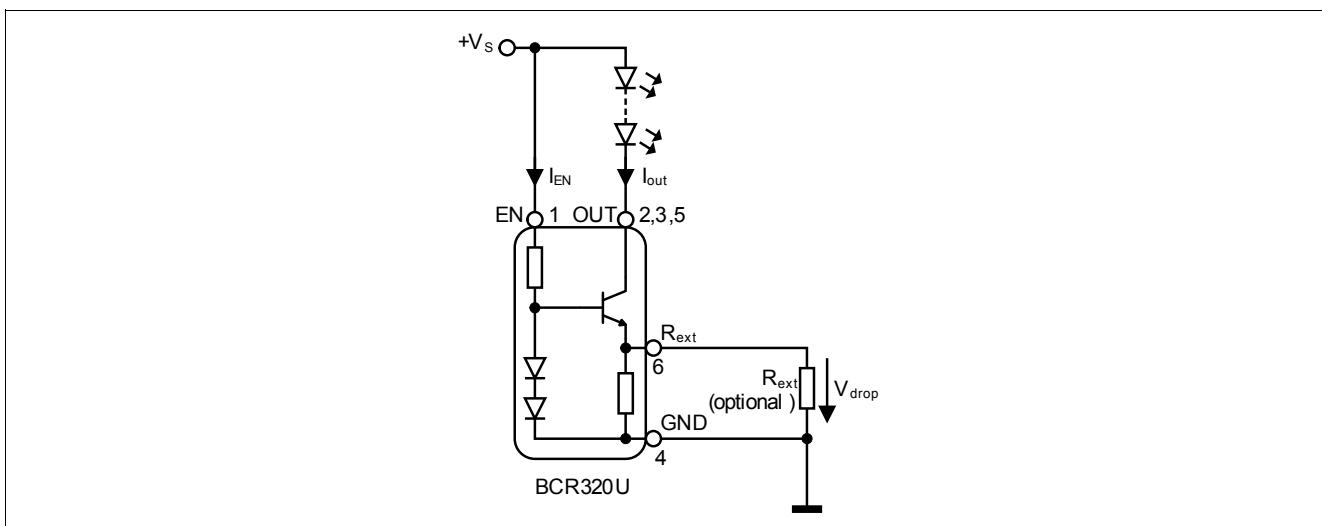
Figure 4-2 Application Circuit: Enabling by Connecting to  $V_s$
