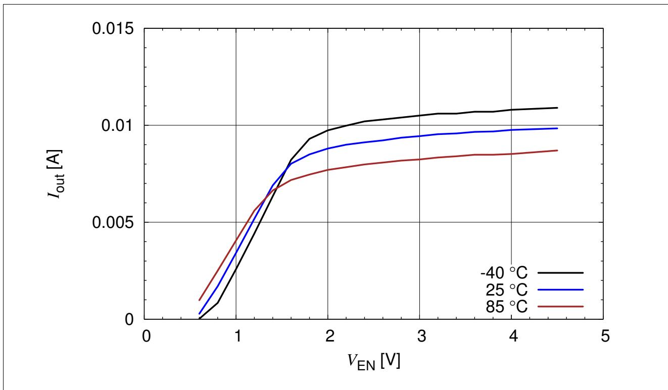
Figure 3-19 BCR321U: Output Current versus  $V_{\text{EN}}$   $I_{\text{out}} = f(V_{\text{EN}})$ ,  $V_{\text{out}} = 2$  V,  $R_{\text{ext}} = \text{open}$ ,  $T_A$  = Parameter
