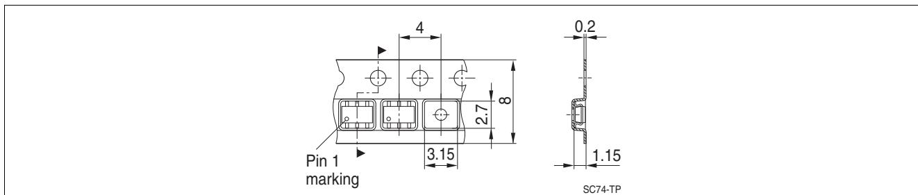
**Figure 5-3 Tape and Reel Information for SC74 (dimensions in mm)**
