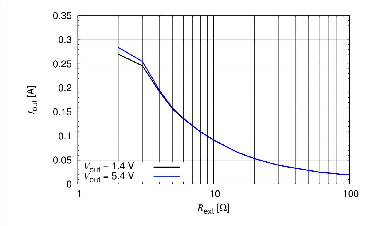
Figure 3-15 BCR321U: Output Current versus  $R_{\text{ext}}$   $I_{\text{out}} = f(R_{\text{ext}})$ ,  $V_{\text{EN}} = 3.3 \text{ V}$ ,  $V_{\text{out}} = \text{Parameter}$
