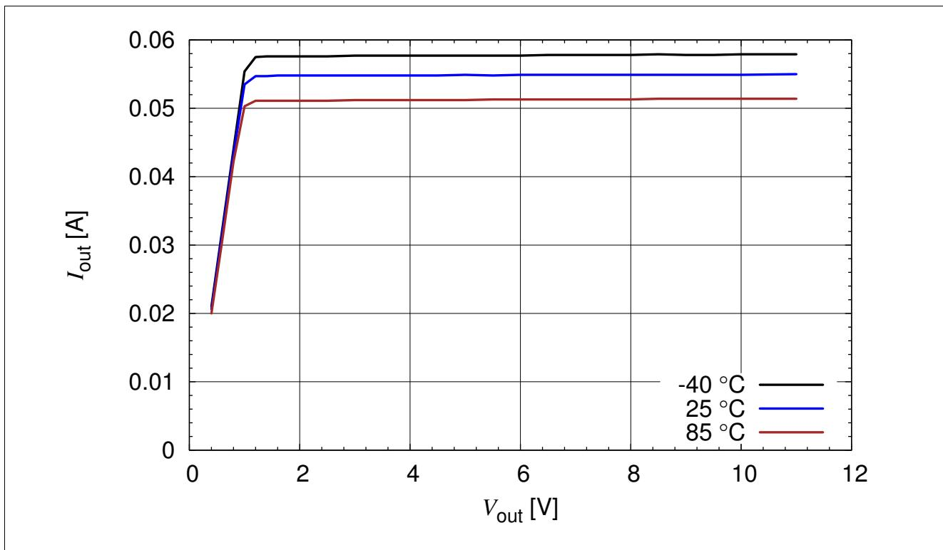
Figure 3-7 BCR320U: Output Current versus  $V_{\text{out}}$   $I_{\text{out}} = f(V_{\text{out}})$ ,  $V_{\text{EN}} = 12 \text{ V}$ ,  $R_{\text{ext}} = 20 \Omega$ ,  $T_A = \text{Parameter}$
