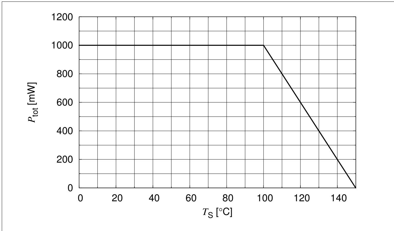
Figure 3-1 Total Power Dissipation  $P_{\text{tot}} = f(T_S)$
