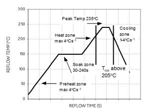
Figure 35. Reflow Profile for Tin/Lead (Sn/Pb) process.
