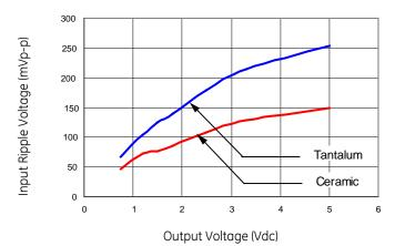
Figure 26. Input ripple voltage for various output with 4x22  $\mu$ F polymer and 4x47  $\mu$ F ceramic capacitors at the input (full load).
