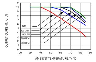
Figure 20. Derating Output Current versus Local Ambient Temperature and Airflow (Vin = 12.0Vdc, Vo=1.8 Vdc).
