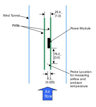
Figure 33. Thermal Test Set-up.
