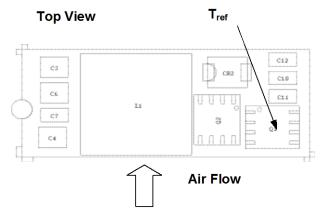
Figure 32. Tref Temperature measurement location.
