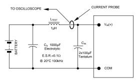
NOTE: Measure input reflected ripple current with a simulated source inductance ( $L_{\text{TST}}$ ) of 1 $\mu$ H. Capacitor C<sub>S</sub> offsets possible battery impedance. Measure current as shown above.
