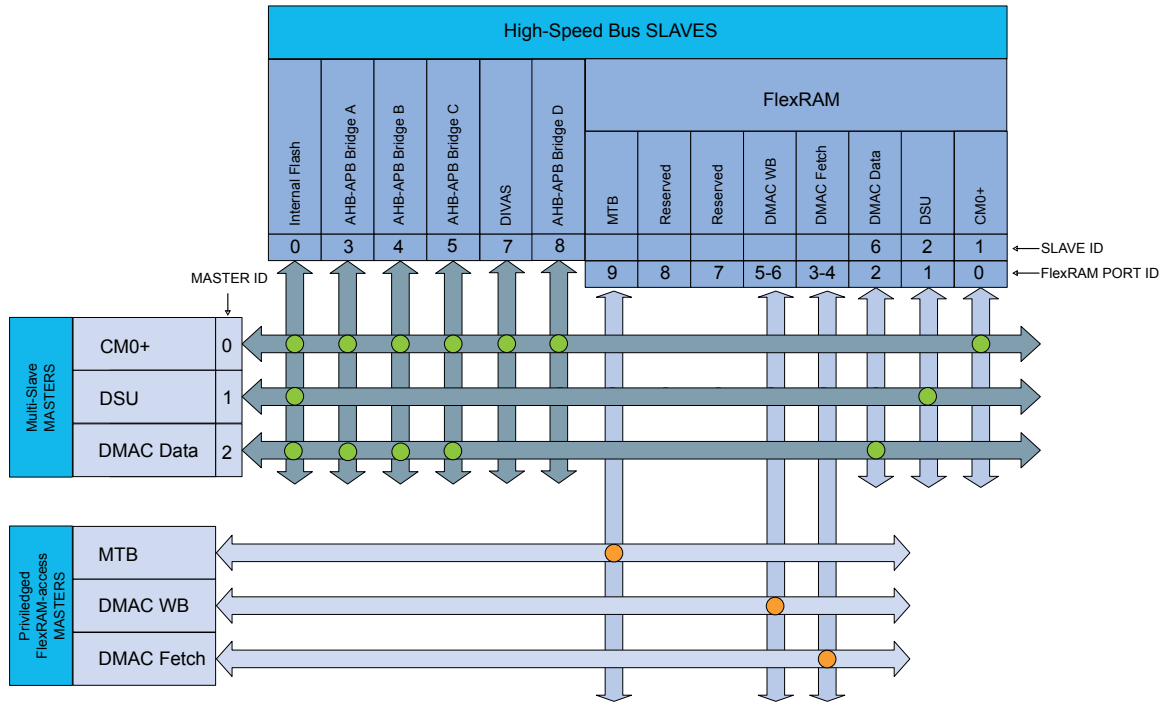
Figure 11-1. Master-Slave Relation High-Speed Bus Matrix (1)
