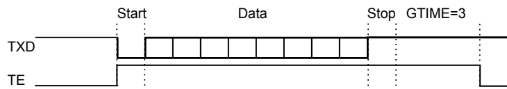
Figure 32-16. Example of TE Drive with Guard Time
