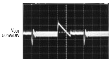
Transient Response (Burst Mode Operation)
