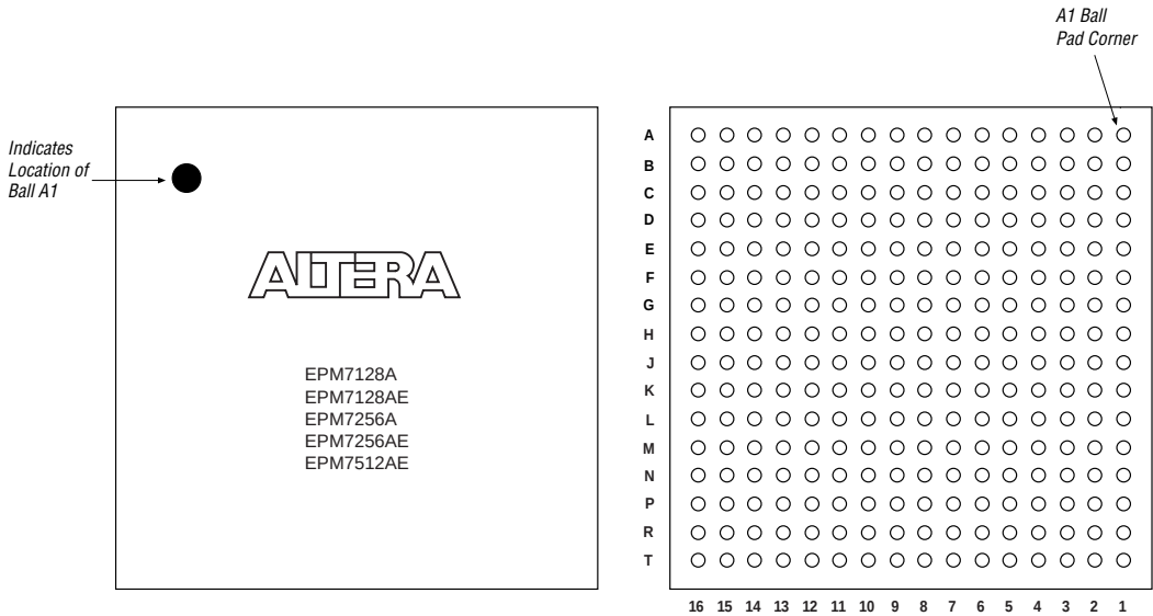
Figure 23. 256-Pin FineLine BGA Package Pin-Out Diagram
