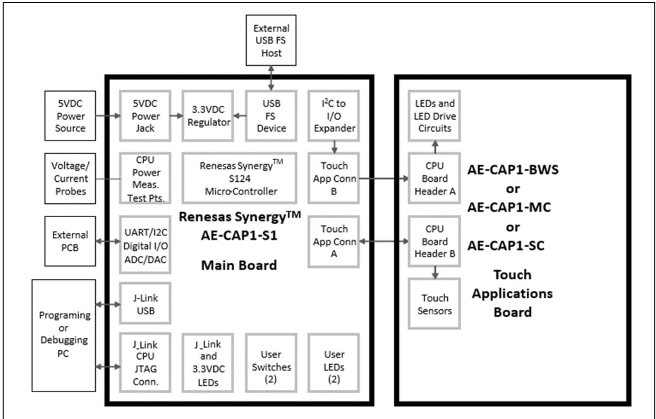
Figure 18 S1 Target Board plus application board
