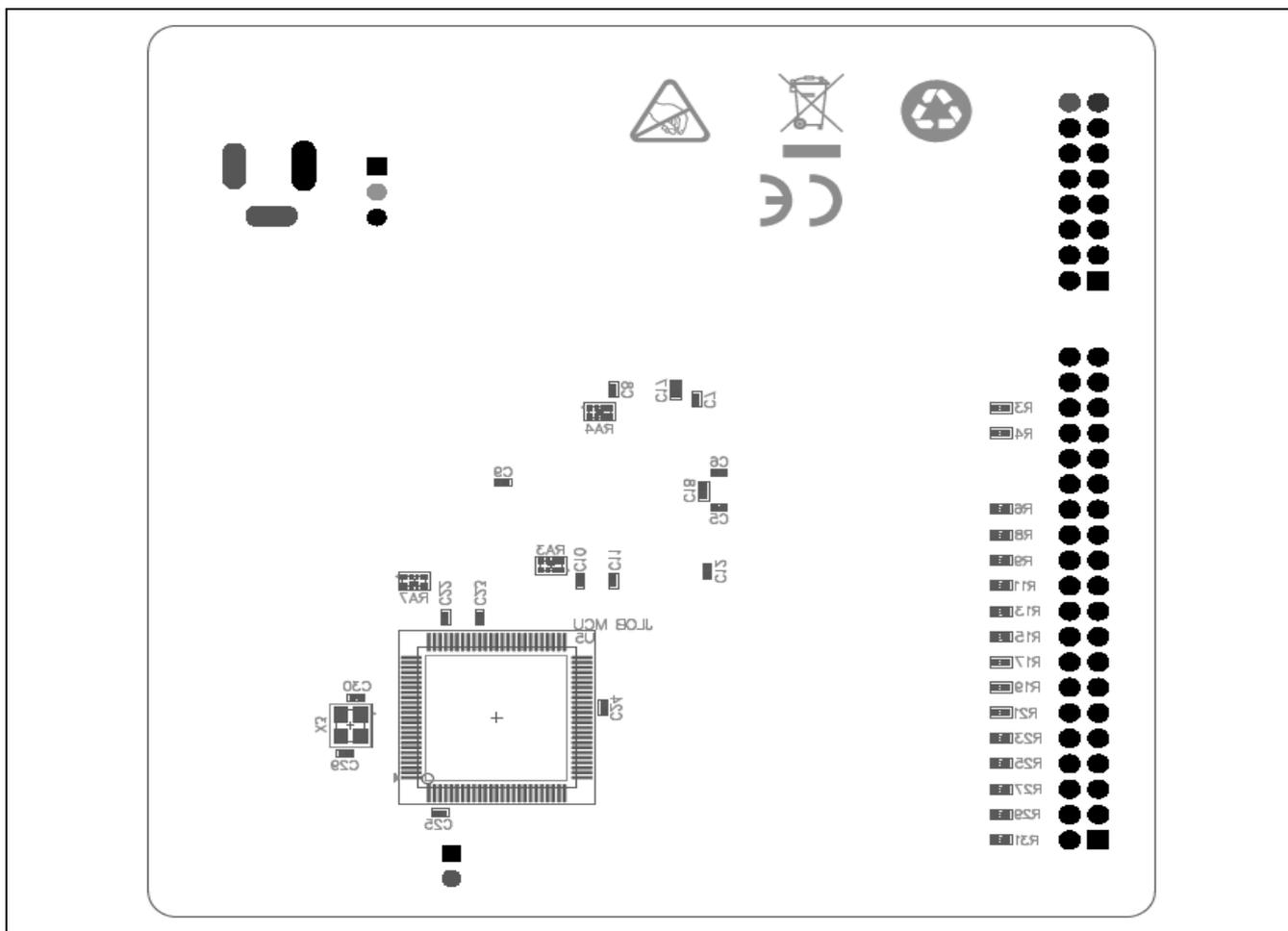
Figure 10 AE-CAP1-S3 Target Board Component Placement, Bottom
