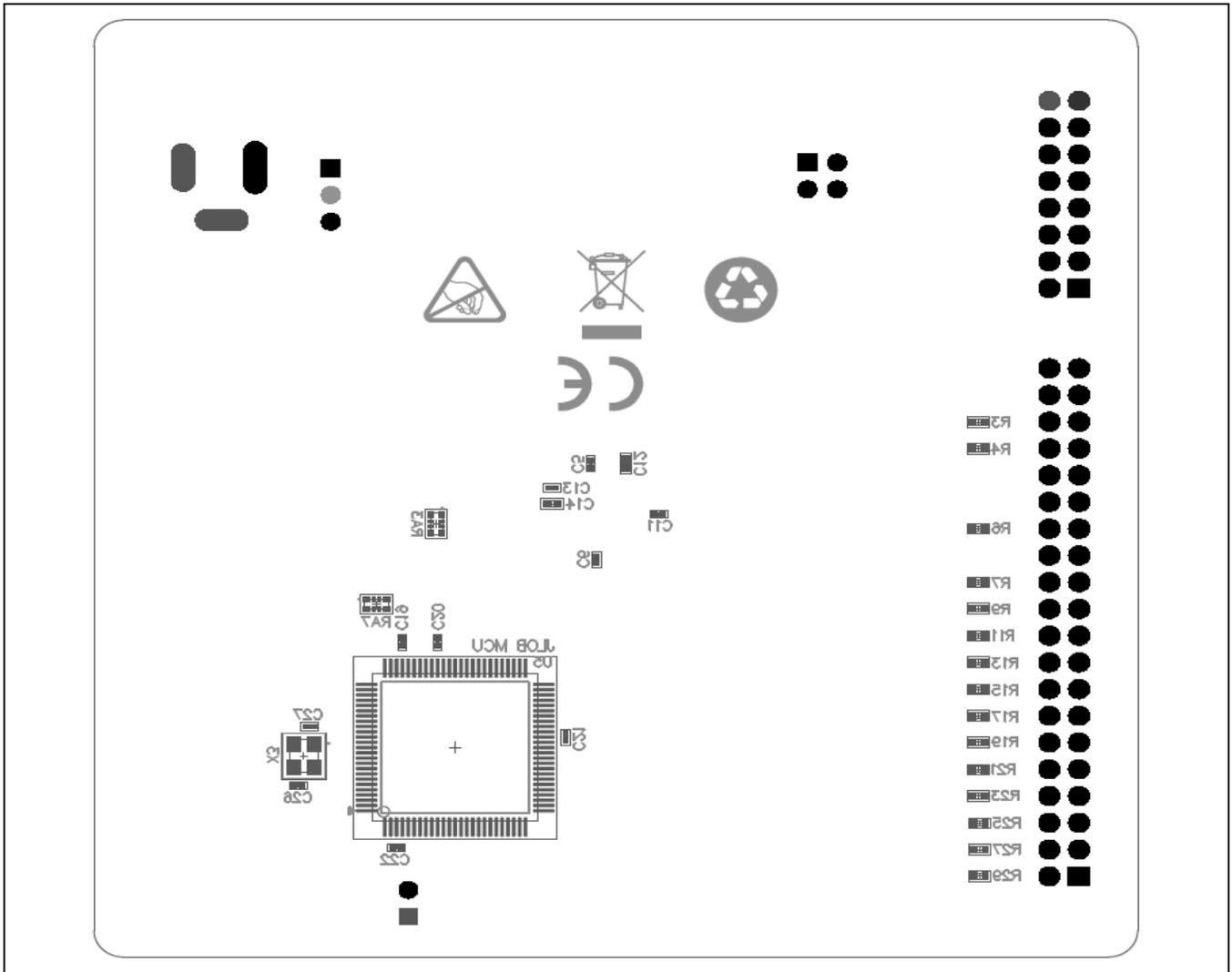
Figure 8 AE-CAP1-S1 Target Board Component Placement, Bottom
