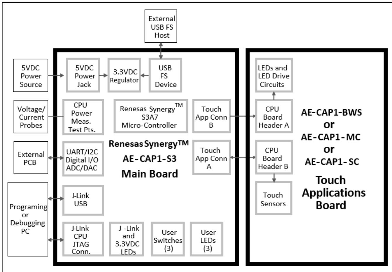
Figure 19 S3 Target Board plus application board
