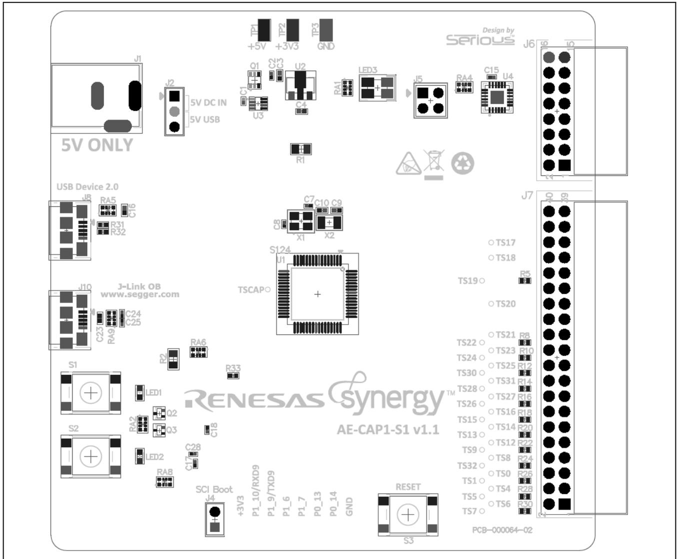
Figure 7 AE-CAP1-S1 Target Board Overall Component Placement, Top
