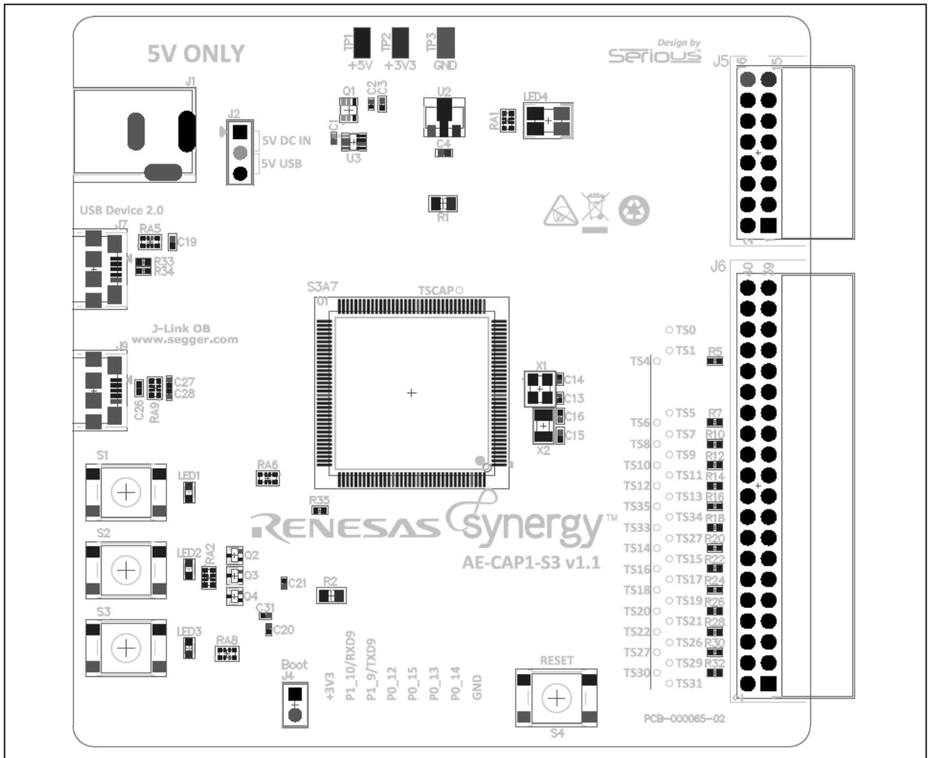
Figure 9 AE-CAP1-S3 Target Board Component Placement, Top
