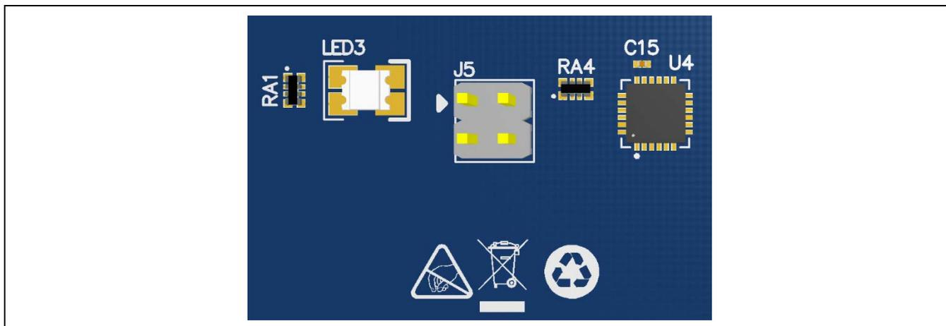
Figure 21 Jumper J5 on AE-CAP1-S1
