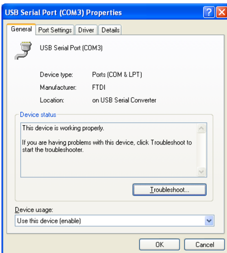
Figure 2.8 – Access COM Port Properties
