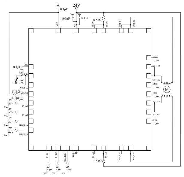
Note: It is recommended that a bypass capacitor is added if necessary. The GND wiring must become one-point-earth as much as possible and designed in consideration with heat dissipation. When the setting pin of each mode is controlled by a switch, pull up or pull down to prevent high impedance state. For input data, refer to the function description.
