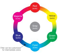
Even for images clearly distinguishable in color, when converted to monochrome the contrast tends to become low. Color filter analyzer automatically selects the optimal color filter (auto color filter) based on the image analysis result to adjust the contrast, to allow for stable image measurement. Any intermediate color can be arranged for the color filter using custom settings.
