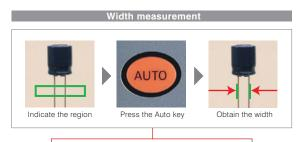
Appropriate filters and edge scan directions for width measurement can be automatically set by analyzing the target image.
