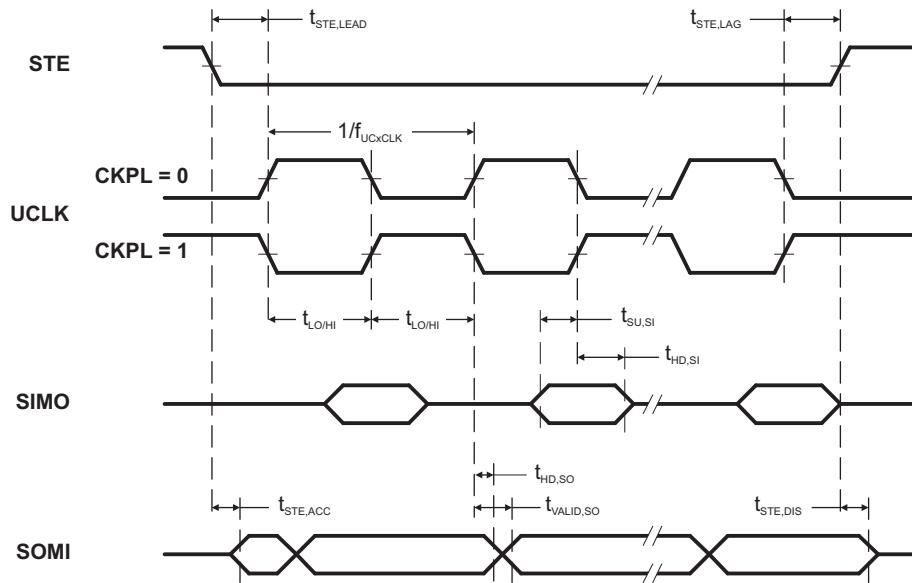
**Figure 13. SPI Slave Mode, CKPH = 0**
