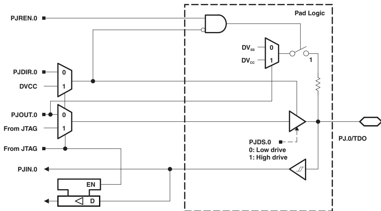
**Port J, J.1 to J.3 JTAG pins TMS, TCK, TDI/TCLK, Input/Output With Schmitt Trigger or Output**
