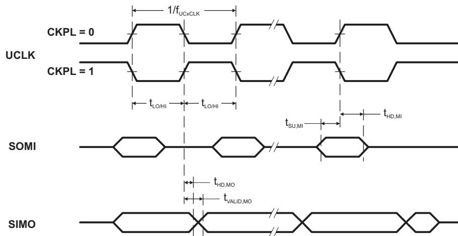
**Figure 12. SPI Master Mode, CKPH = 1**
