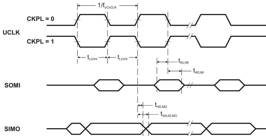
**Figure 11. SPI Master Mode, CKPH = 0**
