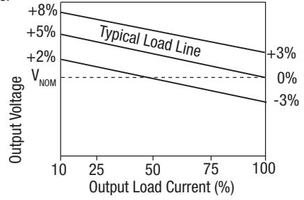
The voltage tolerance envelope shows typical load regulation characteristics for this product series. The tolerance envelope is the maximum output voltage variation due to changes in output loading.
