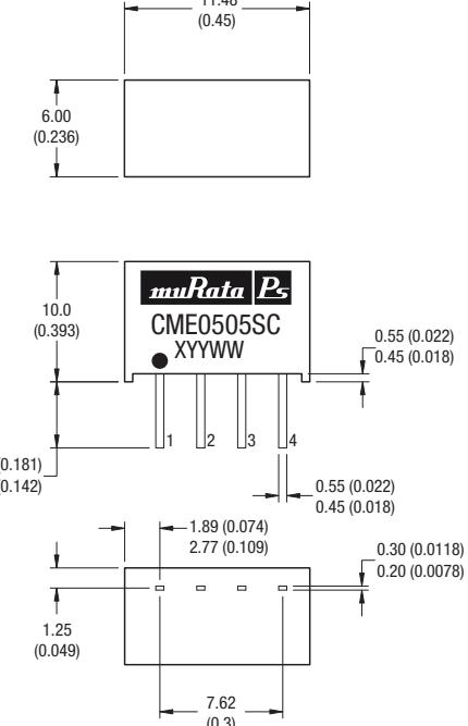
All dimensions in millimetres ±0.25mm (" ±0.01"). All pins on a 2.54 (0.1) pitch and within ± 0.25 (0.01) of true position.
