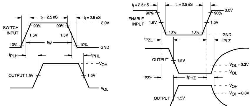
FIGURE 2. AC Waveforms
