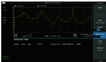
Visualize return loss, reflection coefficient, and VSWR of your DUT.
