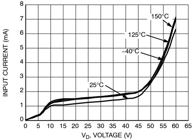
**Figure 16. Input Current vs.  $V_D$  Voltage On-State**
