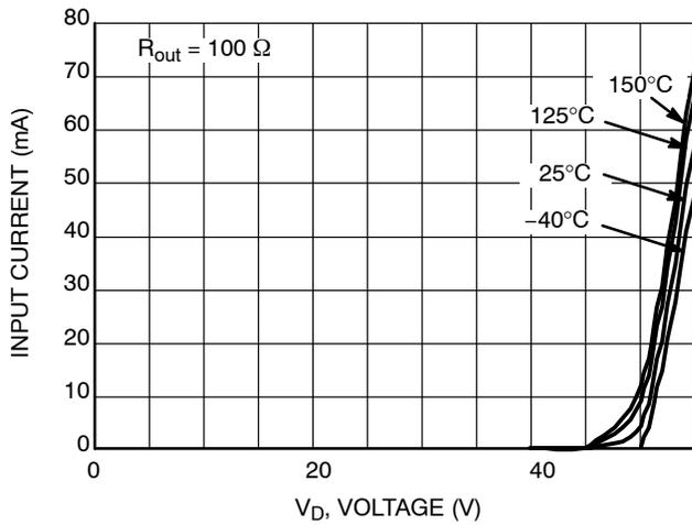
**Figure 18. Input Current vs.  $V_D$  Voltage Off-State**
