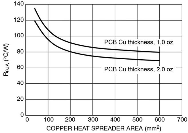
Figure 20. R<sub>θJA</sub> vs. Copper Area
