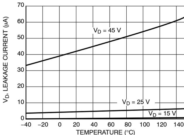
Figure 12.  $V_D$  Leakage Current vs. Temperature Off-State
