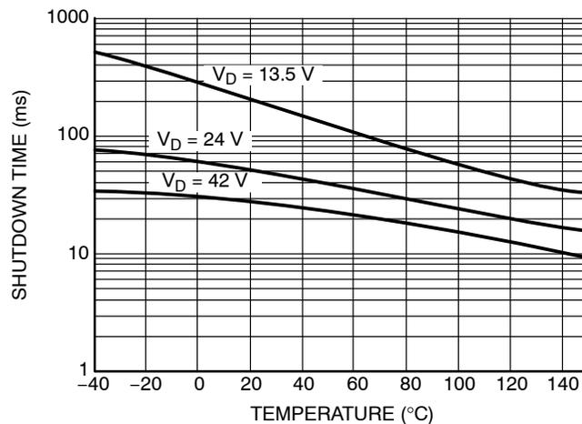
**Figure 19. Initial Short-Circuit Shutdown Time vs. Temperature**
