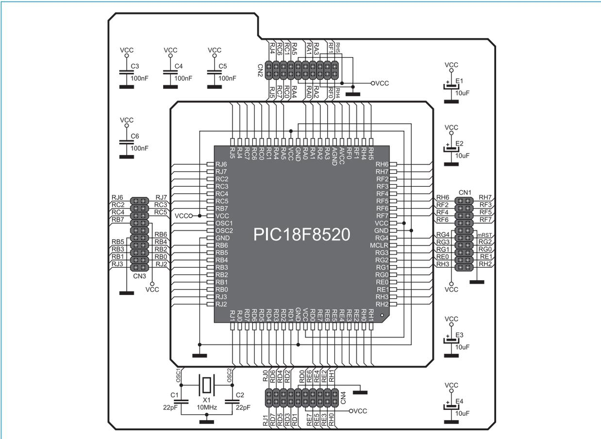
Figure 2: 80-pin MCU card and microcontroller connection schematic
