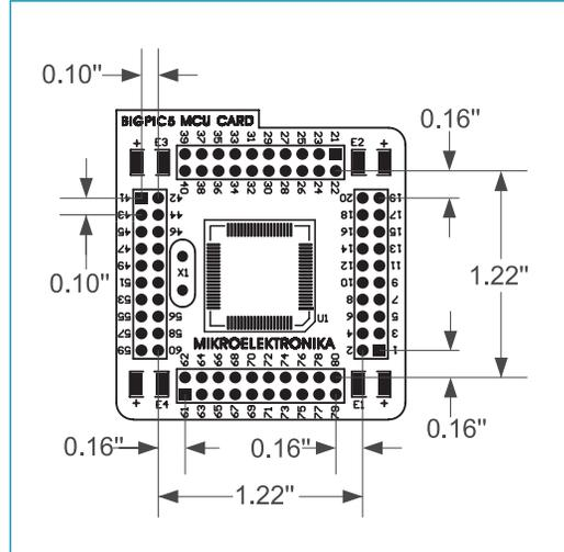
Figure 1-4: Dimensions of MCU card for BIGPIC5
