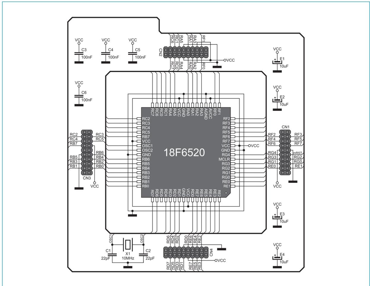
Figure 1: 64-pin MCU card and microcontroller connection schematic
