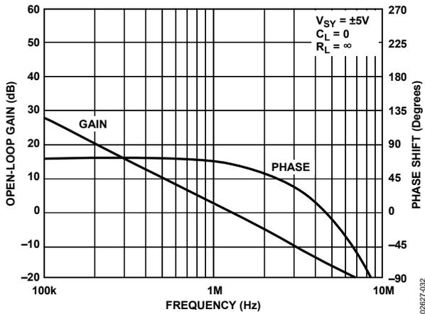
Figure 32. Open-Loop Gain and Phase Shift vs. Frequency
