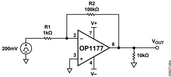
Figure 54. Test Circuit for Overload Recovery Time
