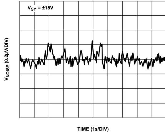
Figure 22. 0.1 Hz to 10 Hz Input Voltage Noise
