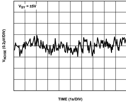
Figure 43. 0.1 Hz to 10 Hz Input Voltage Noise
