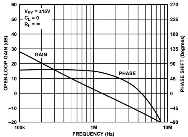
Figure 12. Open-Loop Gain and Phase Shift vs. Frequency
