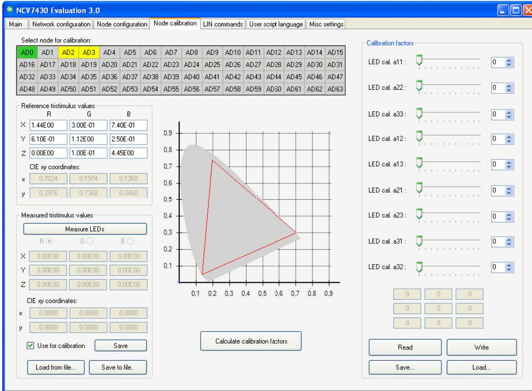
Figure 19. NCV7430 Evaluation – Node Calibration Tab
