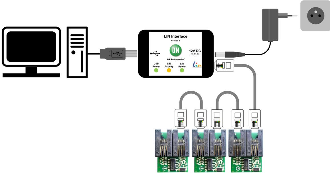
Figure 4. NCV7430 Evaluation Setup Connection (Configuration 1)
