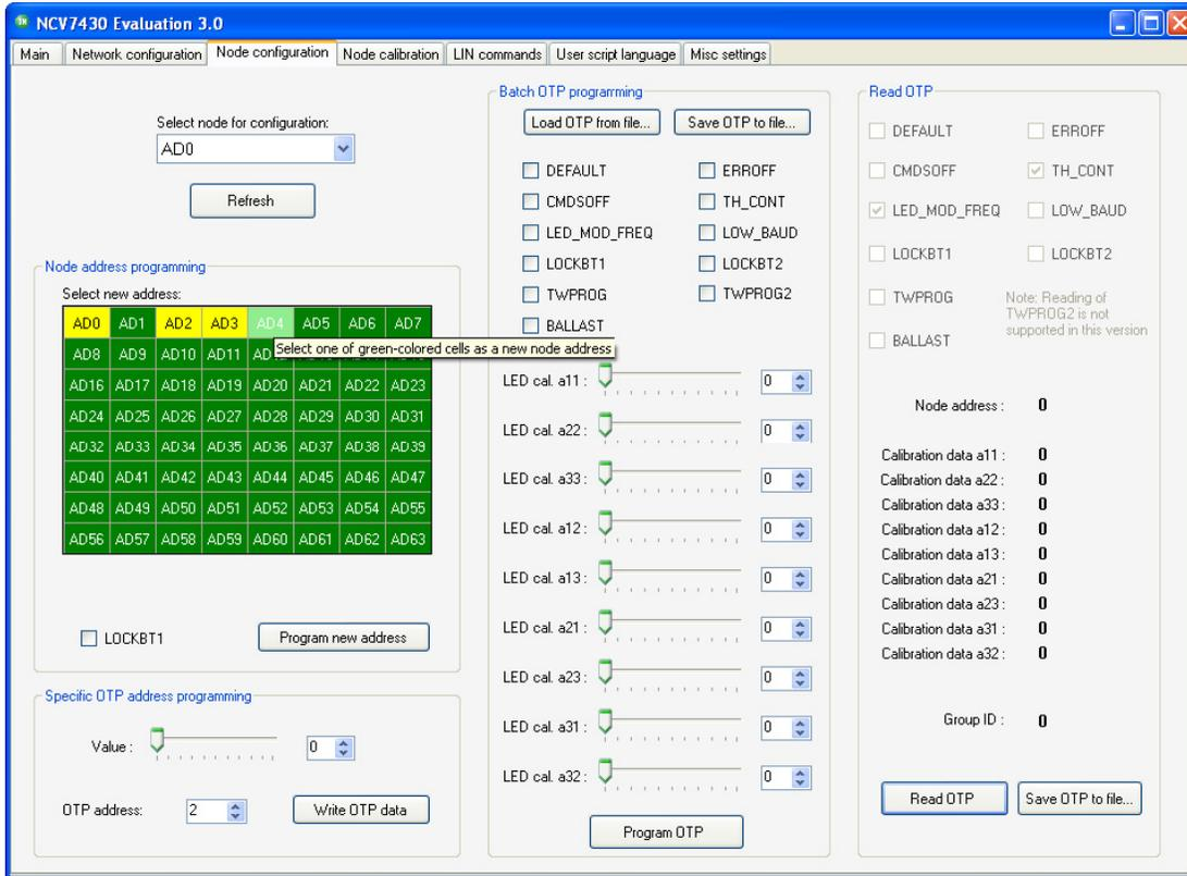
Figure 18. NCV7430 Evaluation – Node Configuration Tab
