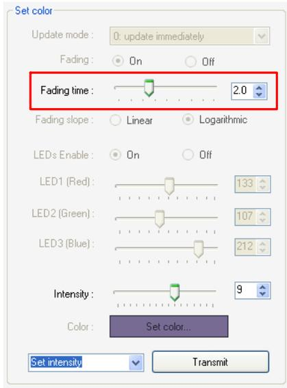
**Figure 14. Set\_Intensity Command**
