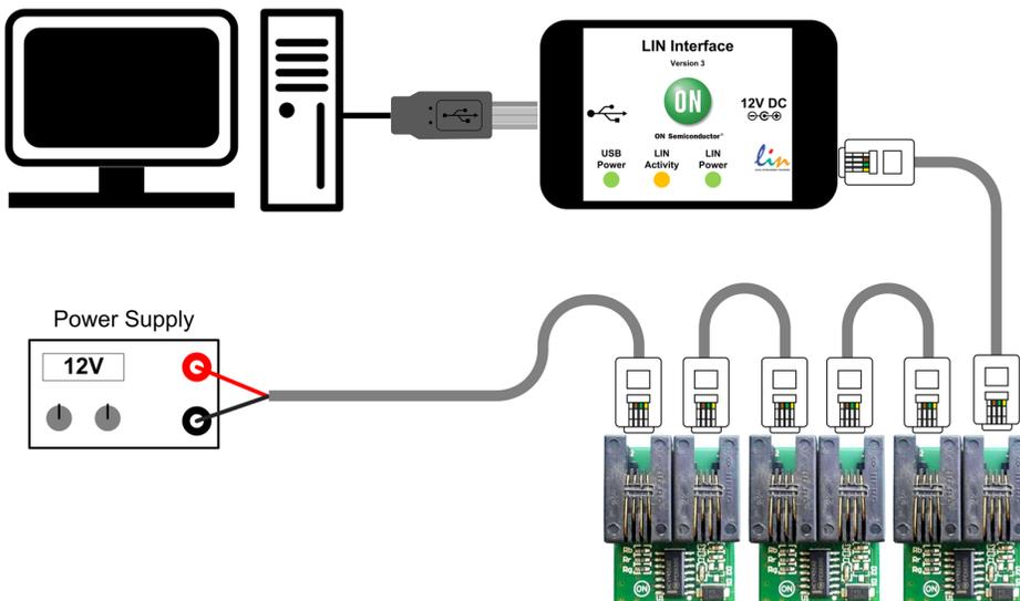
Figure 5. NCV7430 Evaluation Setup Connection (Configuration 2)
