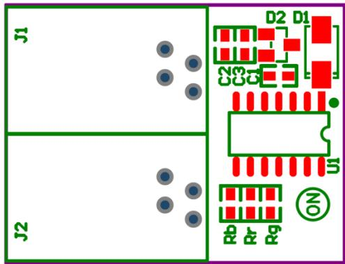
Figure 23. NCV7430 EVB PCB Top Assembly Drawing
