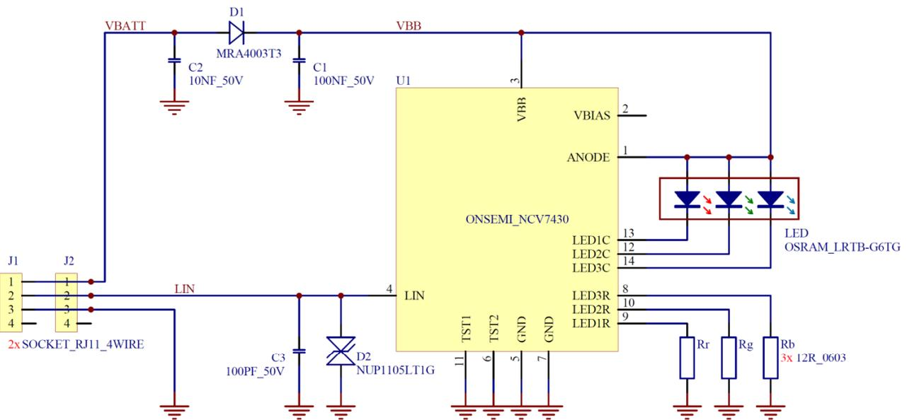
Figure 22. NCV7430 Schematic
