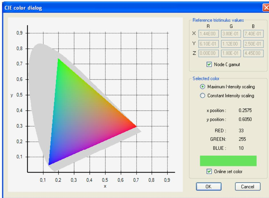
NOTE: With selecting "Online set color", the LED module follows the color chosen in the diagram.
