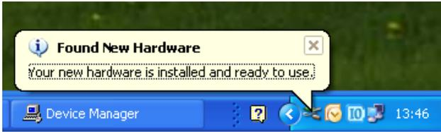
The installation can be checked in Device Manager. When the hardware is connected, you should be able to find *USB Serial Converter A* and *B* in *Universal Serial Bus controllers* group.
