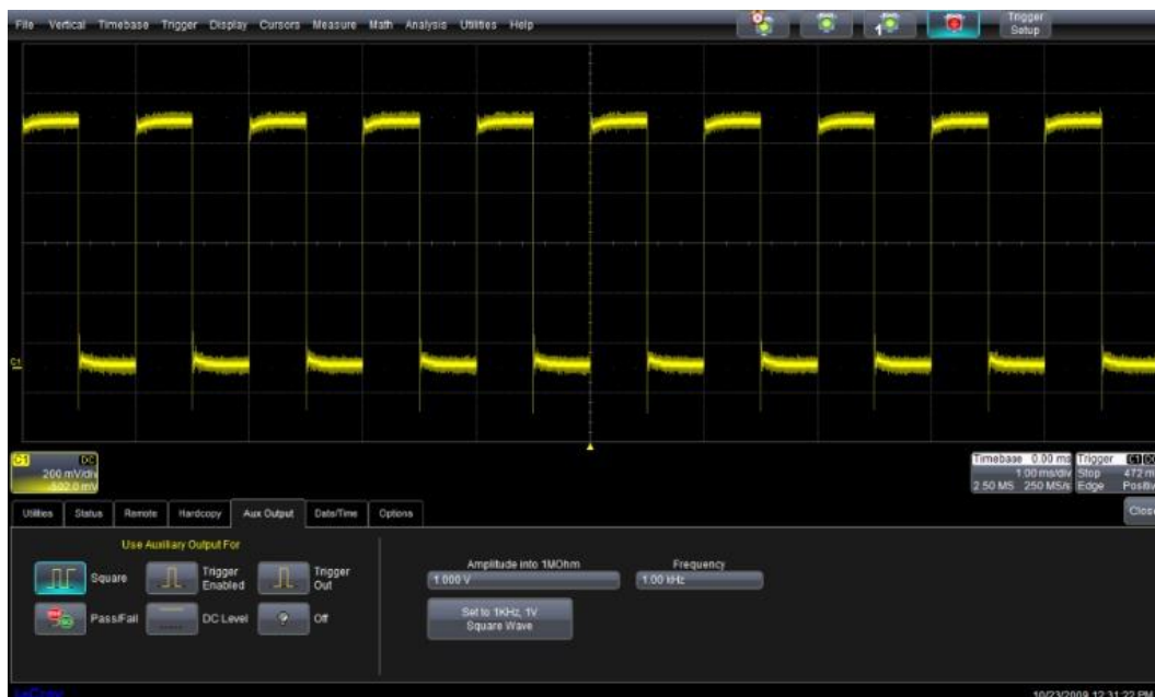
Square wave output signal
