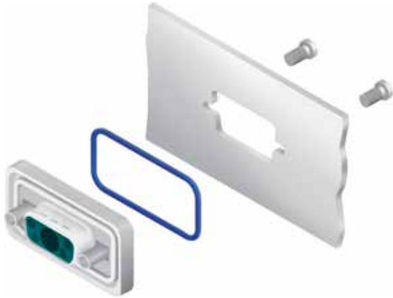
Front panel mounting
