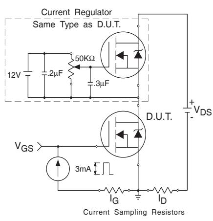
**Fig 13.** Gate Charge Test Circuit
