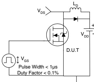
**Fig 14a.** Switching Time Test Circuit
