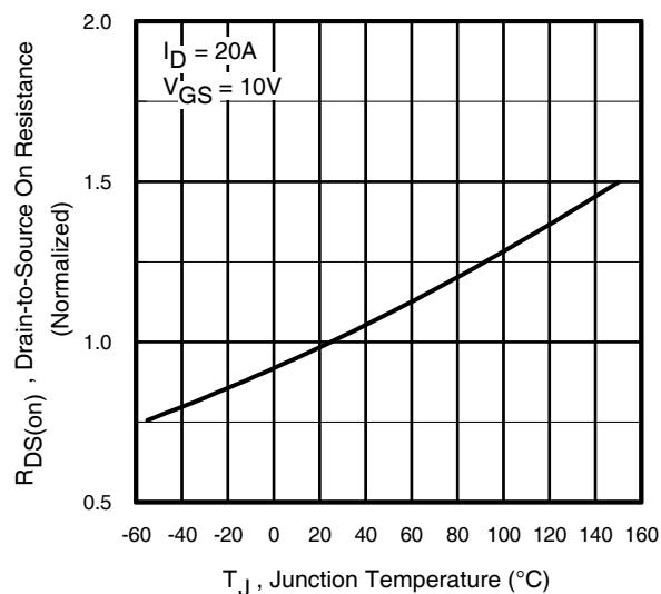
**Fig 4.** Normalized On-Resistance
