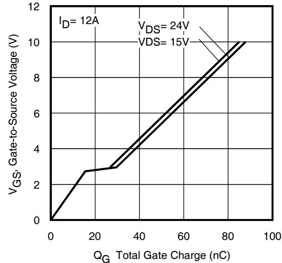
**Fig 6.** Typical Gate Charge Vs.
