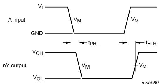
Measurement points are given in [Table 9](#).Logic levels: V<sub>OL</sub> and V<sub>OH</sub> are typical output voltage drop that occur with the output load.**Fig 5. The data input (A) to output (nY) propagation delays****Table 9. Measurement points**
