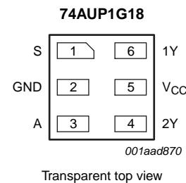
Fig 4. Pin configuration SOT891, SOT1115 and SOT1202
